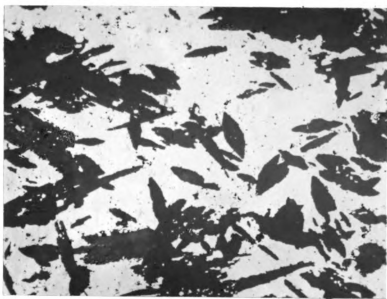
Figure 35.--Random growth of grunerite in magnetite band. Polished surface x80.
