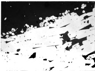
Figure 21.--Typical quartz-specular hematite iron formation member. Note relationship between hematite (white) and magnetite (light gray). Polished surface, x80.
