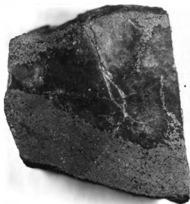
Figure 24.--Rich coarse magnetite vein cutting quartzose layer. Occurrence is typical of intensely folded areas.
