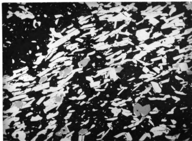
Figure 21.--Typical quartz-specular hematite iron formation member. Note relationship between hematite (white) and magnetite (light gray). Polished surface, x80.
