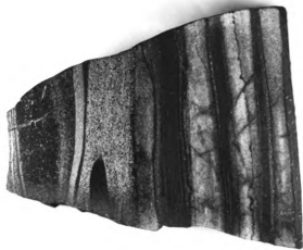
Figure 19.--Contact between banded quartz-specular hematite (left photo) and quartz-magnetite (right photo) iron formation types.
