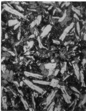
Figure 55.--Diabase Dike.--Lath-shaped plagioclase ( An_{54} ) with interstitial pyroxene (augite).
