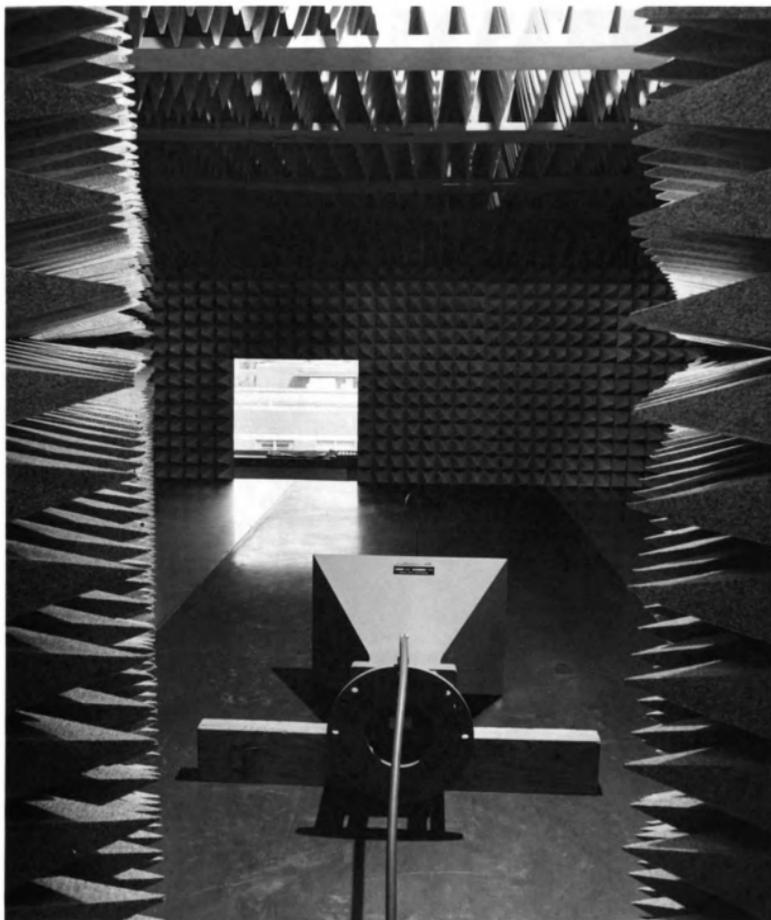
Figure 2.1. Anechoic chamber showing access from rear.
