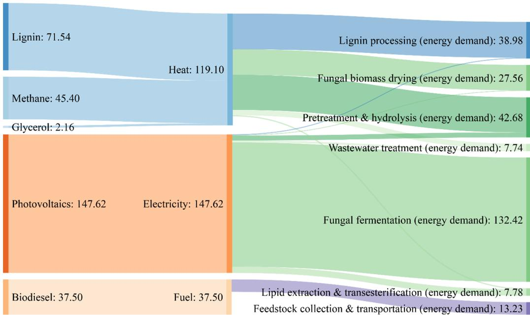
Figure 3-6 Energy balance with Photovoltaic-biological power generation
