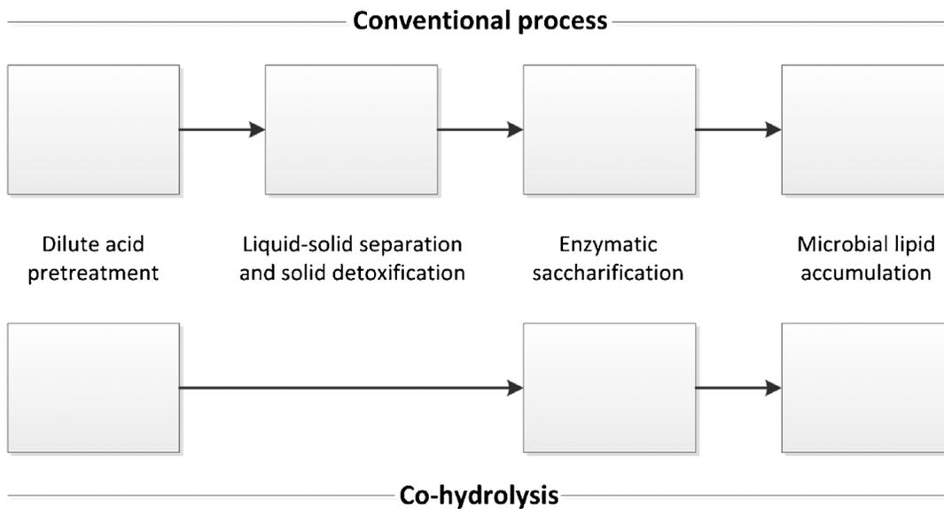
Figure 2-1 Conventional and co-hydrolysis process of dilute acid pretreatment and enzymatic saccharification operation for microbial lipid production (modified from Struder)
