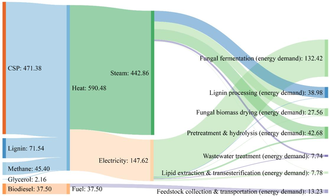
Figure 3-7 Energy balance with concentrated solar power-biological power generation
