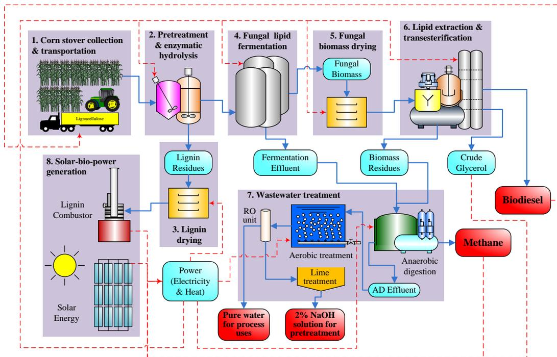
Figure 3-1 Solar-bio-powered lignocellulosic biodiesel refinery mass (blue lines) and energy (red lines) flows
