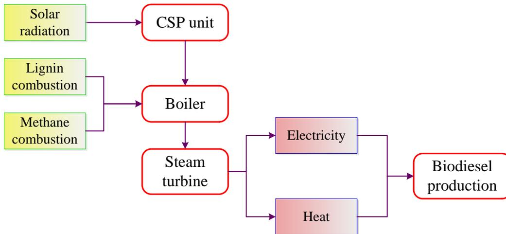
Figure 3-3 Concentrated solar power (CSP) and biological power generation flow diagram
