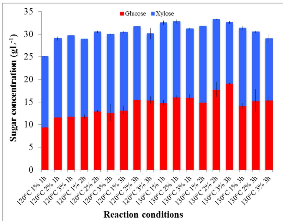
Figure 2-5 Glucose and xylose production from miscanthus under different pretreatment conditions
