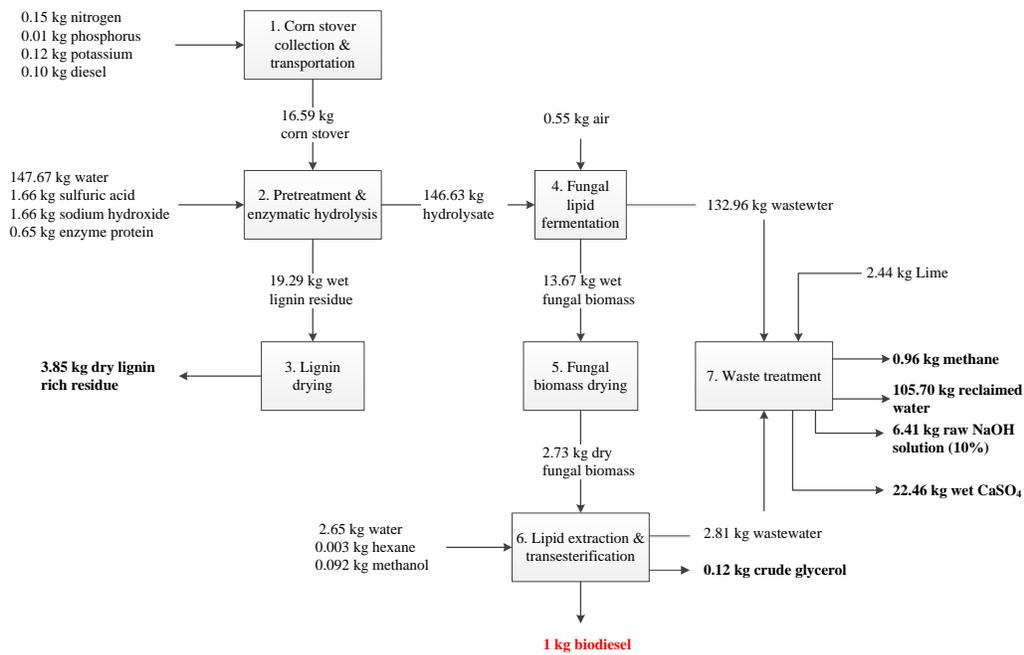
Figure 3-4 Mass flow for the production of 1 kg of fungal biodiesel
