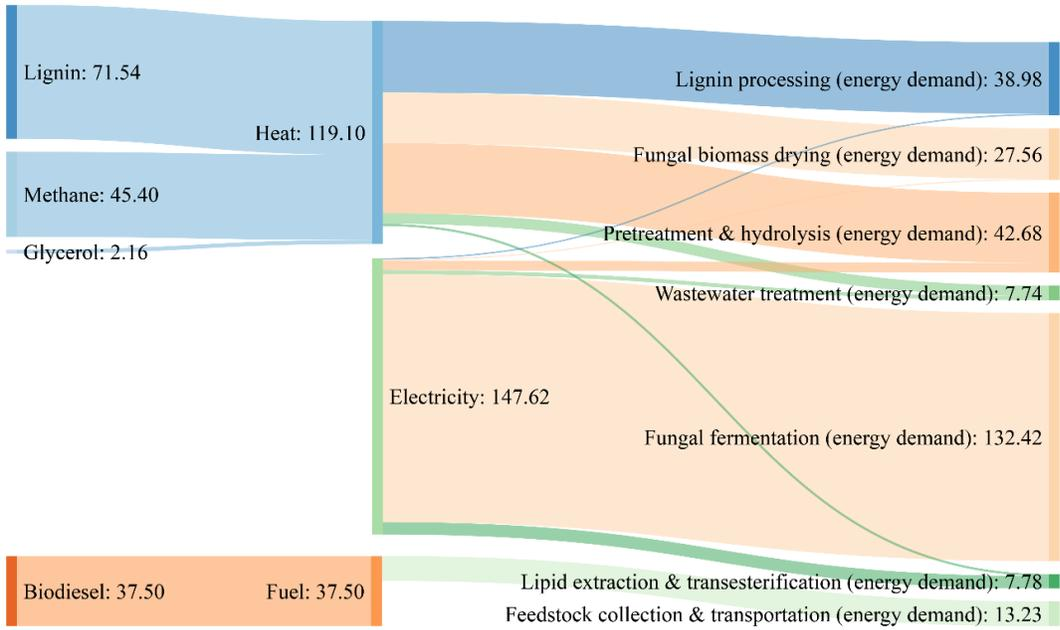
Figure 3-5 Energy balance without solar-bio-power generation
