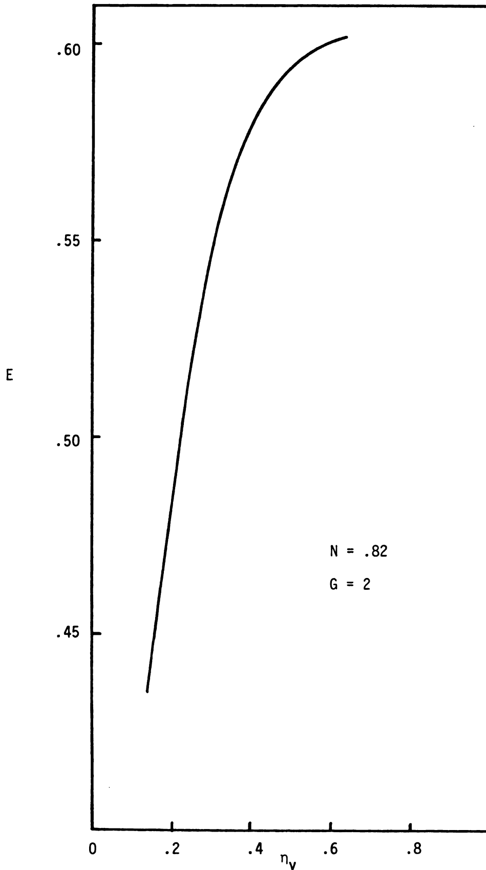
Figure 20.--The Effect of Increasing \eta_v on the Centrifugal Efficiency of a Cylindrical Hydrocyclone.
