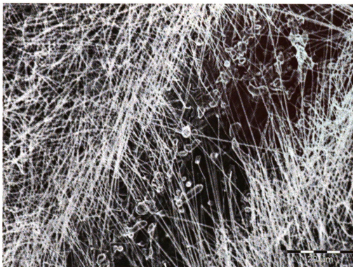
Figure 87. Dark region is no gold zone. The scale bar is 20 \mu\text{m} .
