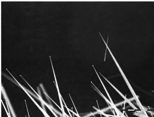
Figure 76. The growth of nanowires on the edge of a silicon wafer. The scale bar is 10\text{ }\mu\text{m} .
