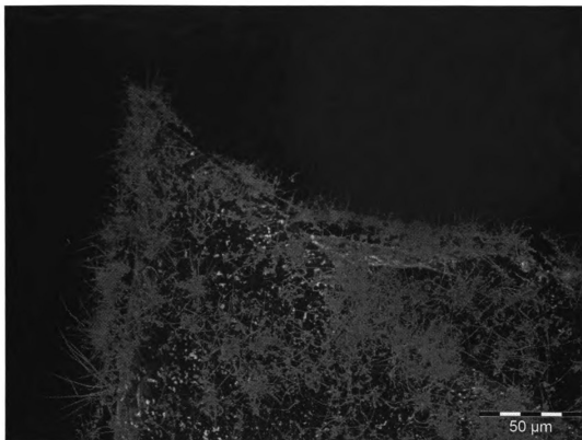
Figure 38. The SEM image of a piece of GaAs. No gold was deposited on this sample before growth.
