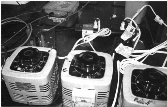
Figure 3-8: Variacs Used for the Test Cells
