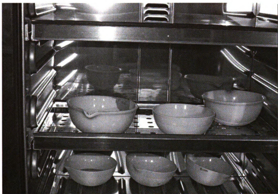
Figure 3-4: Samples kept for Drying in Hot Air Oven
