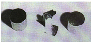
Figure A 9: Bi/Sb (55/45) on W (no LAST), no bond between metals
