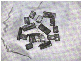
Figure A 1: \text{ZnCl}_2 pre-etch + Sb powder, no bond (out-gassing)
