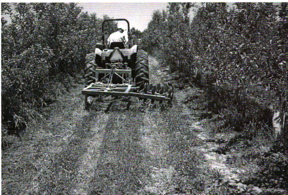
Picture 1: Modified notch disk tiller for the implementation and maintenance of the Sandwich tilled strip.
