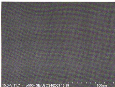
Figure 5-6. SEM image of bare p ++ Si surface.
