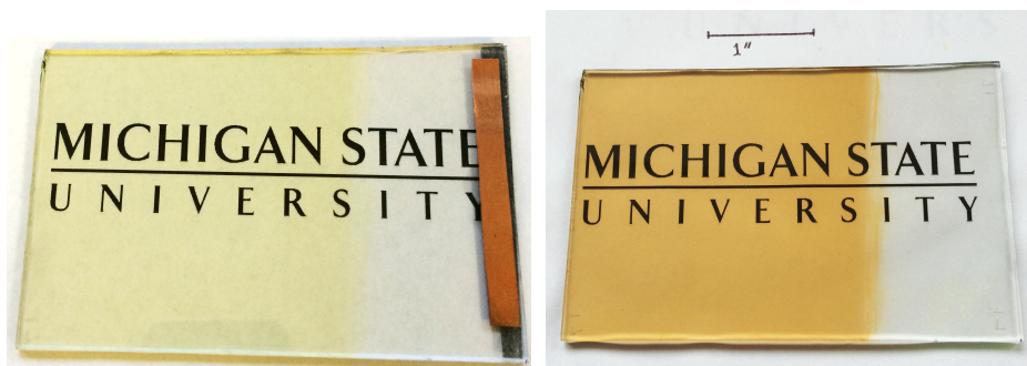
Figure A5-1. Photograph of as-deposited (left) and annealed (right) films prepared via a-ED (deposition time of 60 min).
