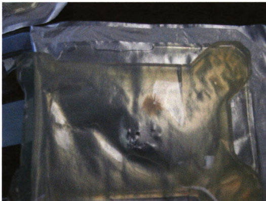
Figure 20 - Test Tray Exhibiting Microbial Growth; Trial Three
