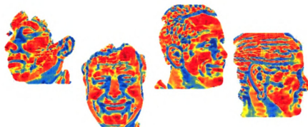
Figure 3.3: Example of the shape index over faces in different poses. Note the consistency of the values around areas such as the eyes and nose regardless of pose.
