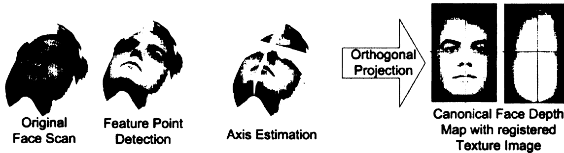
Figure 6.9: Process for generating a Canonical Face Depth Map.
