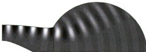
**Figure 7.11** The sound field calculated with the original geometry and without liners applied.
