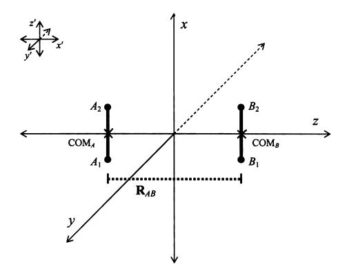
Fig. 13. Parallel arrangement of molecules A and B. In this figure, x, y, and z denote the axes of the laboratory frame, and x', y', and z' denote the axes of the molecular frames of A and B. Also,  $A_1$  and  $A_2$  are the nuclei of molecule A,  $B_1$  and  $B_2$  are the nuclei of molecule B,  $COM_A$  and  $COM_B$  are the centers of mass of molecules A and B, and B, and B is the distance between the center of mass of A and the center of mass of B.
