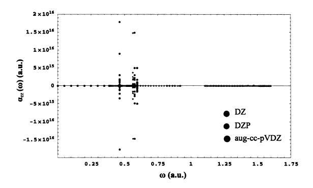
Fig. 6. The zz component of the frequency-dependent polarizability  $\alpha_{zz}(\omega)$  of H<sub>2</sub> as a function of frequency  $\omega$  at the CISD level in the DZ, DZP, and aug-cc-pVDZ basis sets.
