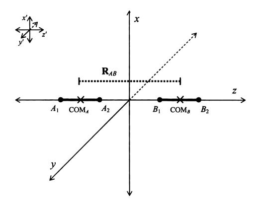
Fig. 12. Colinear arrangement of molecules A and B. In this figure, x, y, and z denote the axes of the laboratory frame, and x', y', and z' denote the axes of the molecular frames of A and B. Also,  $A_1$  and  $A_2$  are the nuclei of molecule A,  $B_1$  and  $B_2$  are the nuclei of molecule B,  $COM_A$  and  $COM_B$  are the centers of mass of molecules A and B, and B, and B is the distance between the center of mass of A and the center of mass of B.
