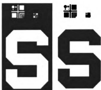
Figure 2-2: Dark field mask (left) and alignment marks (top left). Clear field mask (right) and alignment marks (top right).
