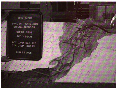
Figure 68. Flexure-Shear Failure of SCC3 Shear Test Unit
