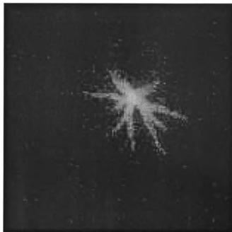
Figure 4.7. Corona at the beginning of an ignition event.
