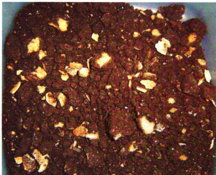
Figure 5.20 Sample 9A PHB-Kenaf composites-End of study image
