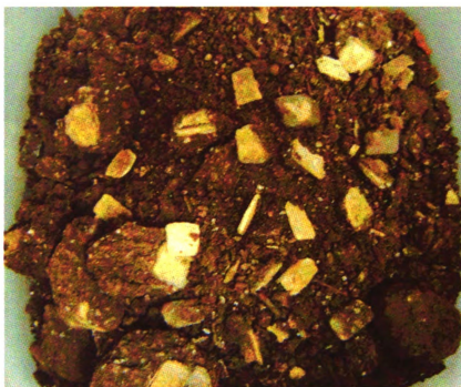
Figure 5.19 Sample 3A PHB-Kenaf composites-End of study image
