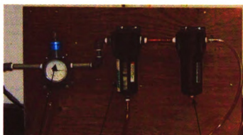
Pressure regulator Air Filter Desiccant-Air dryer
