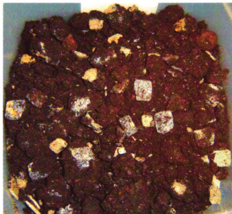
Figure 5.24 Sample 10A PHB-g MA-PHB-Kenaf composites-End of study image
