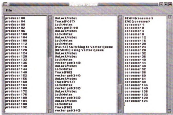
Figure 4.6: Adaptive queue example application. The left pane is the producer, the right the consumer and the center represents status information. Note the Pause and Resume messages where the array-based queue is exchanged with a vector-based queue by the control thread.
