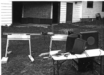
Figure 9.13. Through-lossy-dielectric slab image scene where the S-band rail SAR is located 29.5 feet from the slab.
