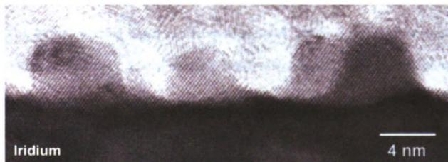
**Figure 5.19** HRTEM image of Ir surface for a  $t_b = 60$  min,  $t_g = 0$  min sample showing the Ir pillars [154].
