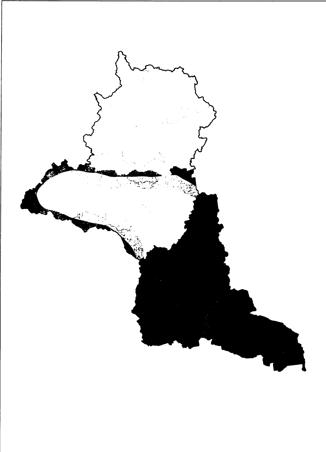
Figure 16. GIS sub-watershed delineation of the Rifle River watershed, Michigan. Upper, middle, and lower sub-watersheds comprise 31%, 30%, and 39% of the total watershed area respectively.
