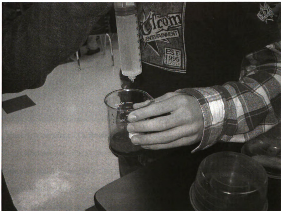
Figure 2: Titration of Remaining 0.25\text{M Ba(OH)}_2 with 0.01\text{ M HCl}
