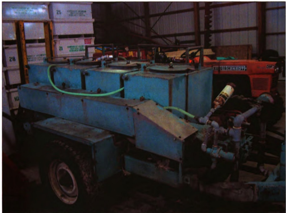
Figure 1.A. Custom built research plot sprayer with a JBS model 705 hand gun, used to apply fungicides for efficacy trials at the Northwest Horticultural Research Station.
