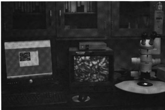
Figure 3 – From Left to Right, Dell Dimensions 4550 Computer, Sony Camera Adapter CMA-D2 on Top of a Sony Trinitron, and a Leica MZ 12 Stereomicroscope Attached to a Computer. Sigma Scan Pro 5.0 Program is on Screen of Computer. Michigan State University, Forensic Anthropology Laboratory.
