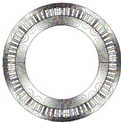
(c) Magnetizing flux pattern for 80% 9-phase voltage and 20% 3-phase voltage.
