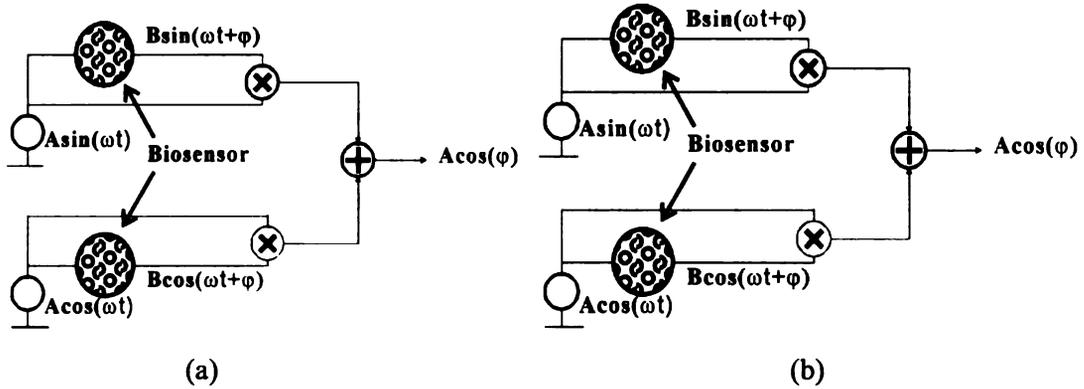
Figure 3.7. The principle block diagram of the fast interrogation EIS system: (a) the configuration to produce the real portion of the admittance, (b) the configuration to produce the imaginary portion of the admittance.
