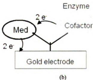
Figure 1.4. Biosensor platform with soluble protein immobilized.
