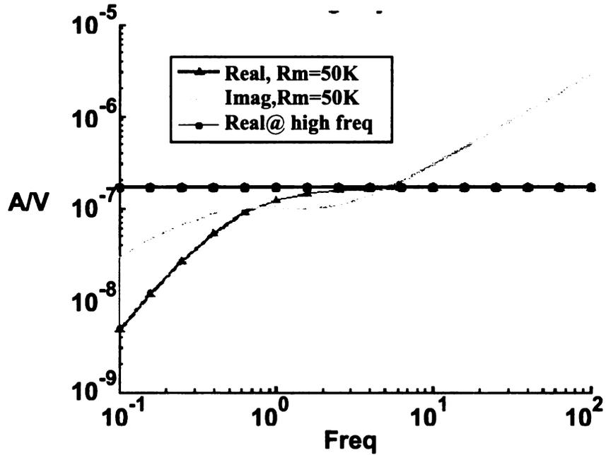
Figure 3.12. A plot of the real and imaginary admittance of a tBLM biosensor model.
