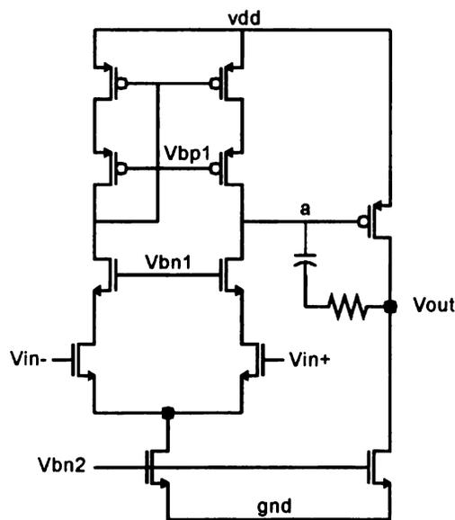
Figure 2.6. Schematic of the two stage amplifier.
