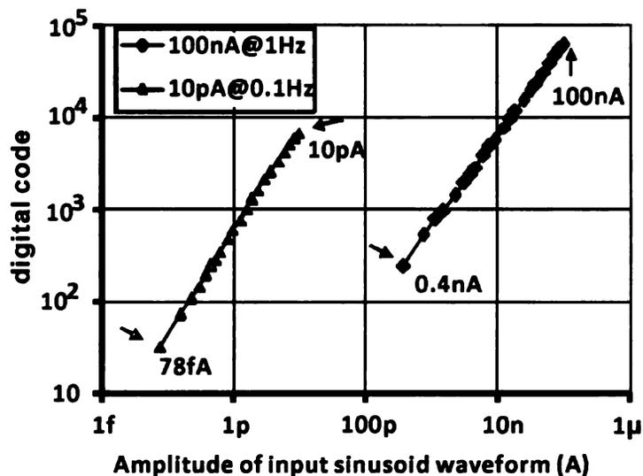
Figure 6.5. Amplitude conversion characterization for the zero phase sine wave input. The lock-in ADC is configured to accommodate a wide range of input signals.
