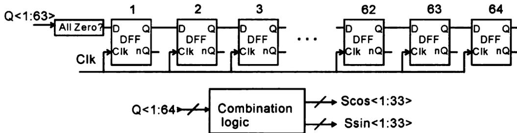
Figure 5.22. The token ring based switch network's control signal generator.
