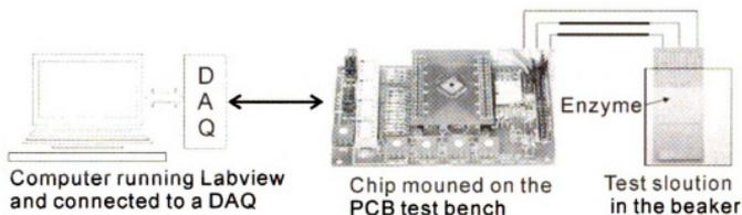
Figure 2.9. The testing setup for the biosensor microarray based on-chip platform.
