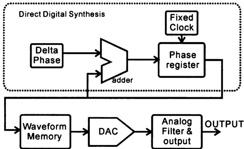
Figure 5.2. The block diagram of the direct digital synthesis based signal generator.
