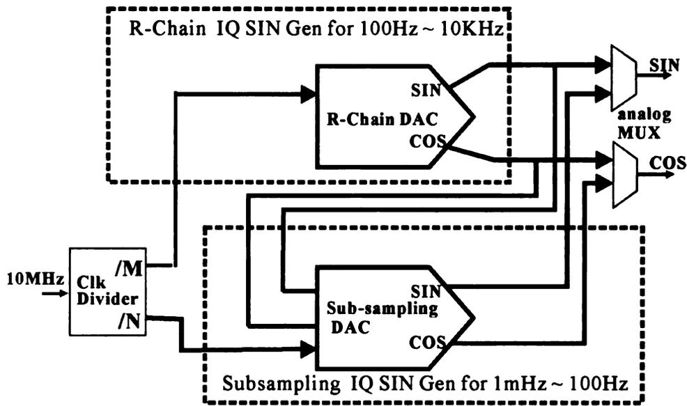
Figure 5.4. The principle structure for the proposed quadrature signal generator.
