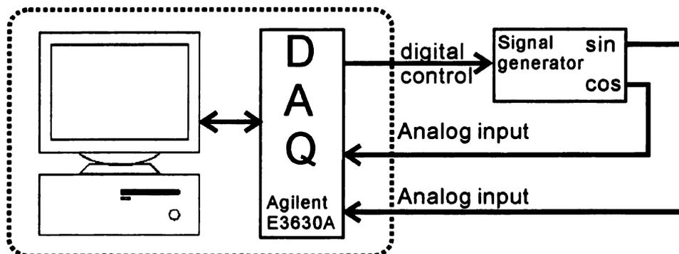
Figure 6.10. Experiment setup for the signal generator testing.
