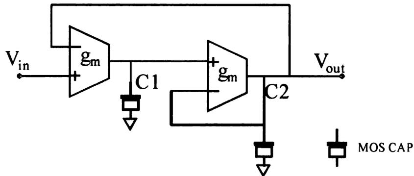
Figure 5.12. Schematic of the  $g_m$ -C biquadratic filter.
