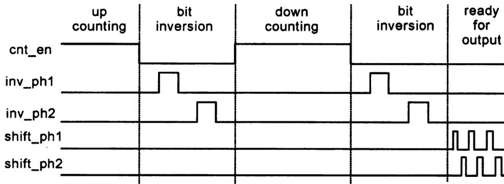
Figure 4.17. Waveform of the control signals for the proposed bidirectional counter/shifter.
