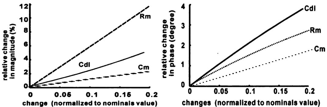
Figure 3.10. Magnitude and phase changes due to a change of up to 20% in component values found in the tBLM biosensor circuit model. The base values for the components are  $R_m=50K\Omega$ ,  $C_m=0.5\mu F$  and  $C_{dl}=5\mu F$ .
