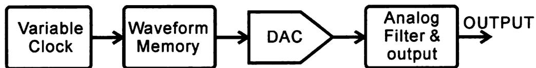
Figure 5.1. The block diagram of the variable clock based digital domain signal generator.
