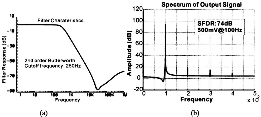
Figure 5.18. (a) Transfer function and (b) the linearity of the variable filter with a cut-off frequency of 250Hz.
