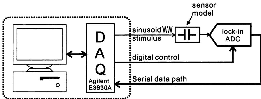
Figure 6.2. Experiment setup for the lock-in ADC.
