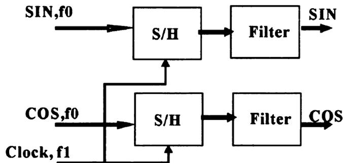
Figure 5.10. The block diagram of a sub-sampling system.
