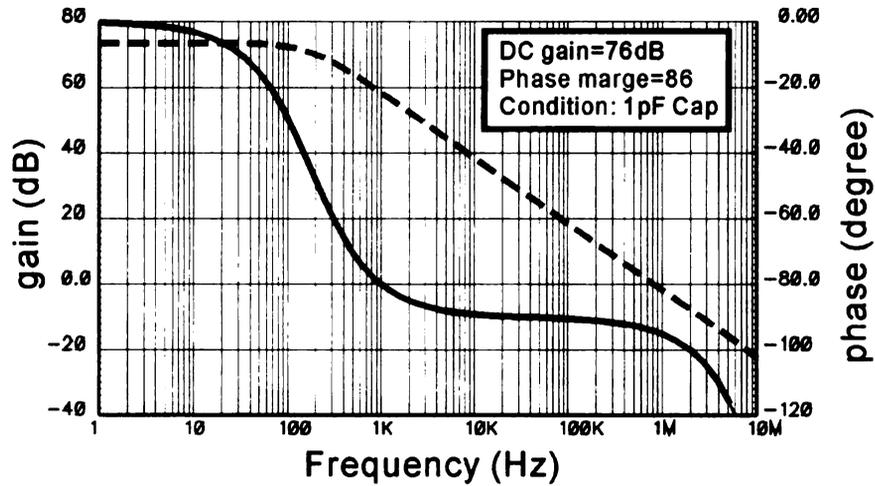
Figure 4.13. AC simulation of the amplifier in Figure 4.12.
