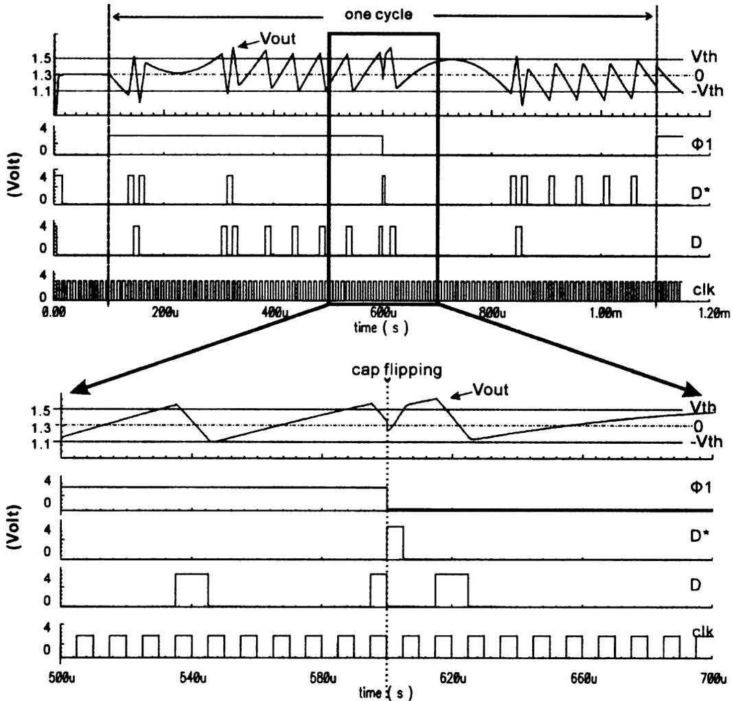
Figure 4.20. The simulation waveforms of some signals in the lock-in ADC system. The input sinusoid stimulus frequency is 1kHz.
