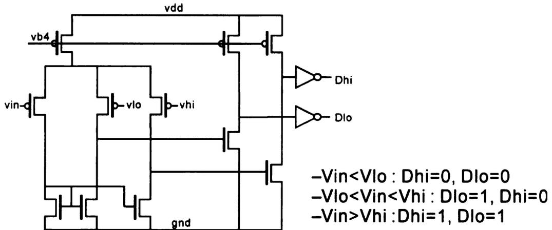
Figure 4.14. Circuit schematic of a dual-level comparator.
