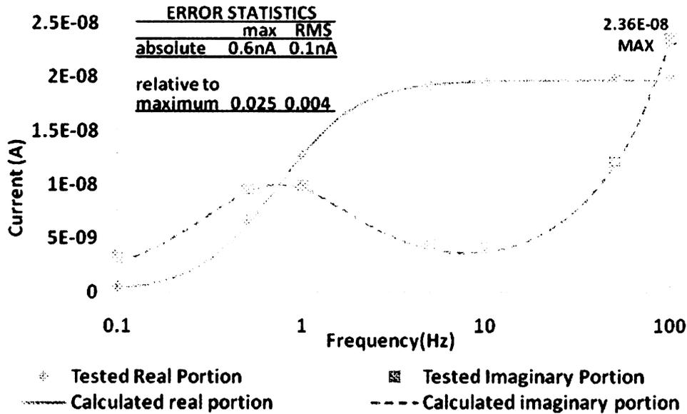
Figure 6.7. The real and imaginary coefficients of current response from the setup in Figure 6.6. The test result and theoretical expectations are given for comparison.
