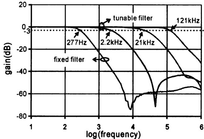
Figure 6.11. Measured frequency response of the filters on the signal generator chip.
