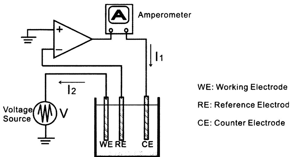
Figure 2.1. Simplified schematic of a typical electrochemical potentiostat system. Normally three electrodes are employed: a working electrode, a reference electrode and a counter electrode.
