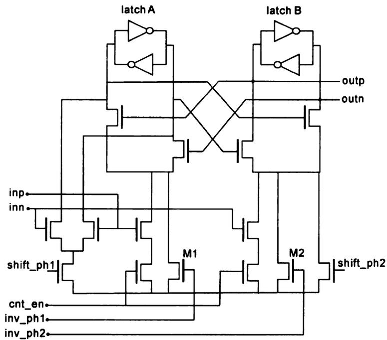
Figure 4.16. Schematic of the new up/down counter with shift register capability.
