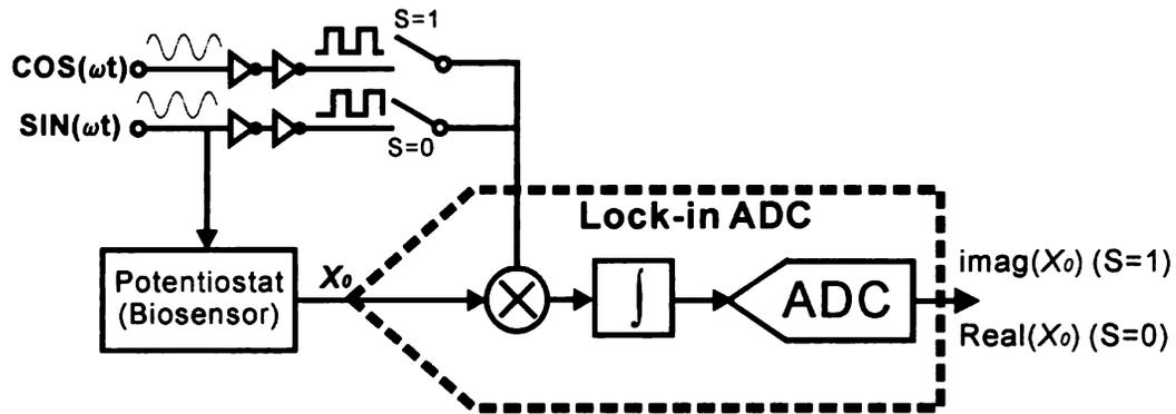
Figure 4.3. Functional block diagram of the proposed EIS system.
