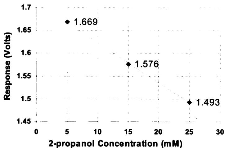
Figure 2.11. Oxidation peak values VS. 2-propanol concentration levels.
