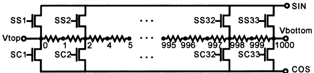
Figure 5.11. A circuit for an R-chain DAC for a signal generator.
