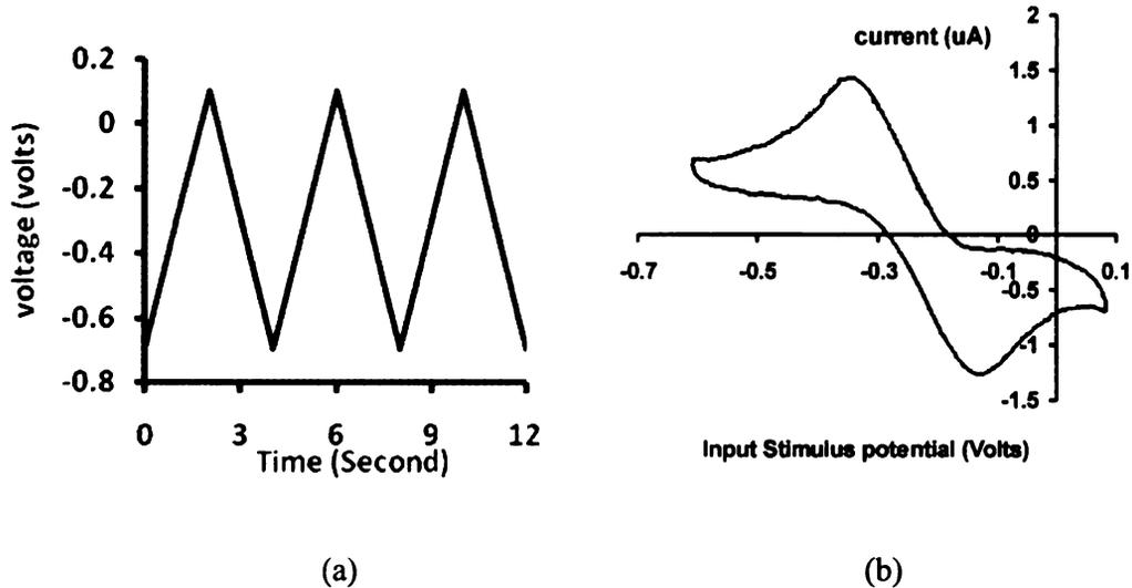
Figure 2.2. (a) typical stimulus potential for cyclic voltammetry, (b)cyclic voltammogram.
