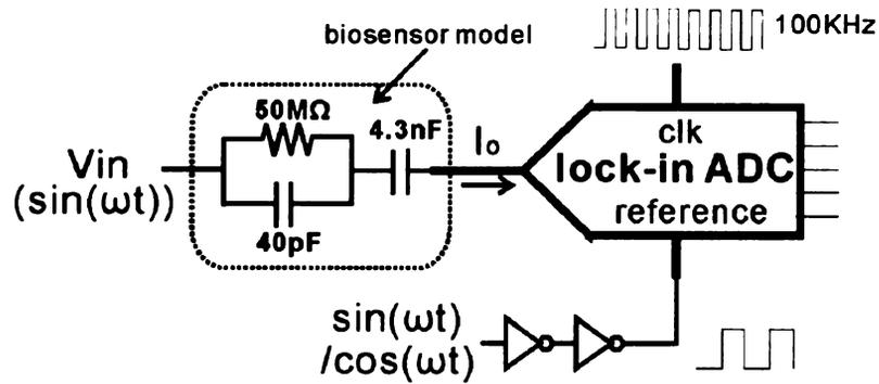
Figure 6.6. Experiment setup for verifying impedance extraction.
