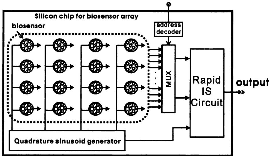
Figure 3.8. The principle block diagram of the fast EIS microsystem.
