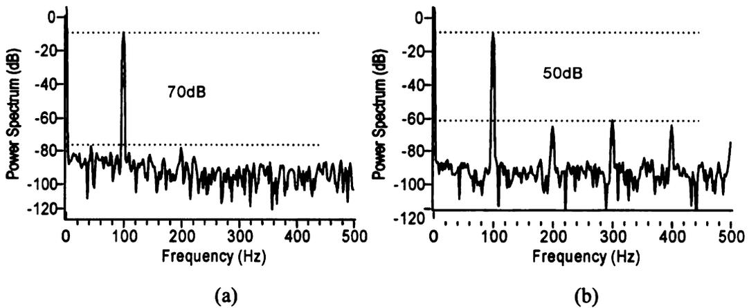
Figure 6.12. Output spectrum for a 100Hz sine input with a 450mV amplitude for (a) a tunable filter and (b) a fixed filter.
