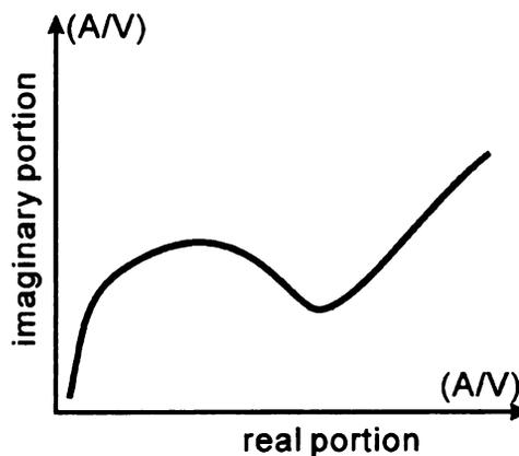
Figure 2.4. Example of the Nyquist plot of the admittance for a biochemical potentiostat.
