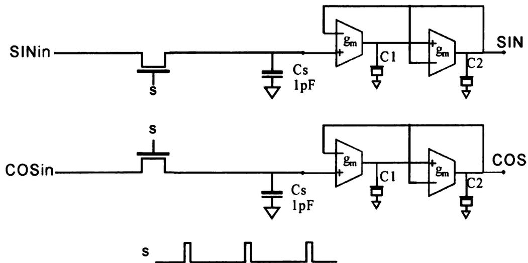
Figure 5.19. Circuit of the sub-sampling quadrature sinusoid signal generator.
