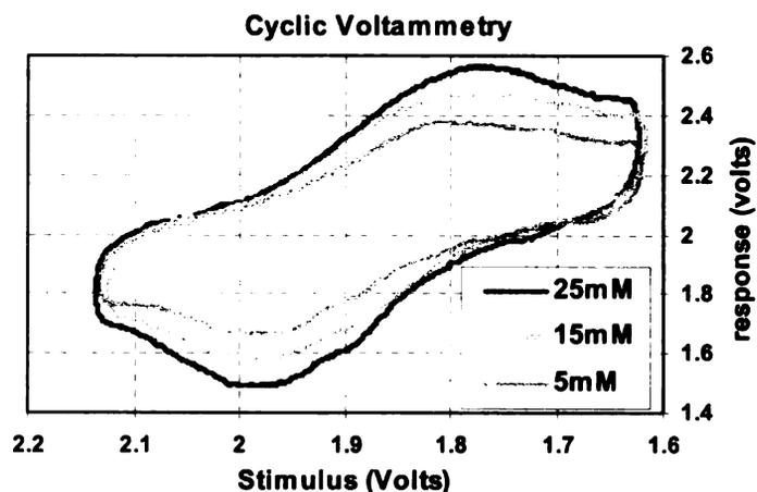
Figure 2.10. Cyclic voltammogram of secondary alcohol dehydrogenase modified electrodes in 5, 15 and 25 mM 2-propanol in 0.1M PBS, at 25 ° C and 100mVs<sup>-1</sup> scan rate, vs. Ag/AgCl reference electrode.
