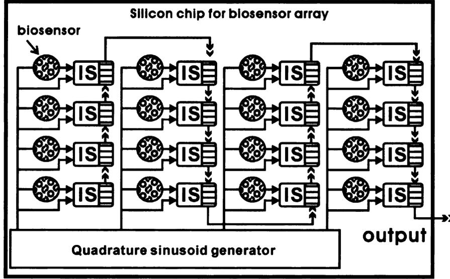
Figure 3.11. The principle block diagram of the multi-channel EIS microsystem.
