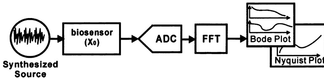
Figure 3.3. The principle block diagram of FFT based EIS system.
