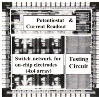
Figure 2.8. Die photograph of the 2.3x2.2mm CMOS chip with surface electrodes and circuit blocks labeled.
