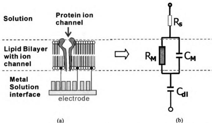
Figure 3.1. (a) structure of the tBLM biosensors and (b) their equivalent circuit model.
