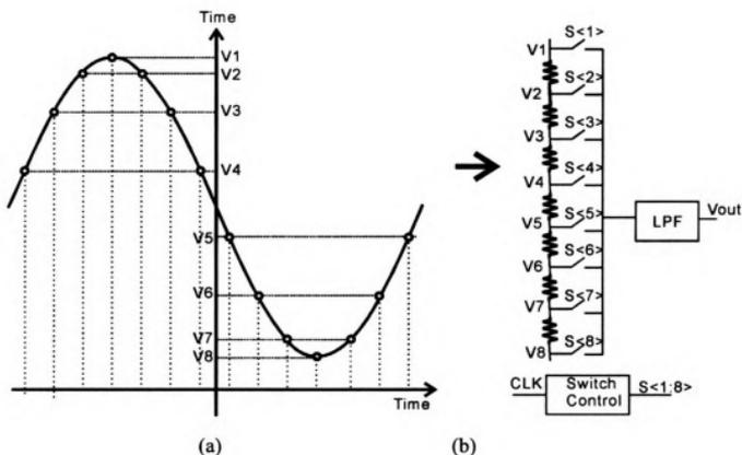
Figure 5.5. Example of a resistor chain based DAC working as sinusoid signal generator (oversampling ratio is 14), (a) the sampling points in a sinusoid waveform; (b) the structure of a DAC with an unevenly tapped resistor chain.
