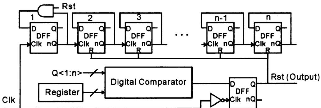
Figure 5.20. The clock divider circuit.
