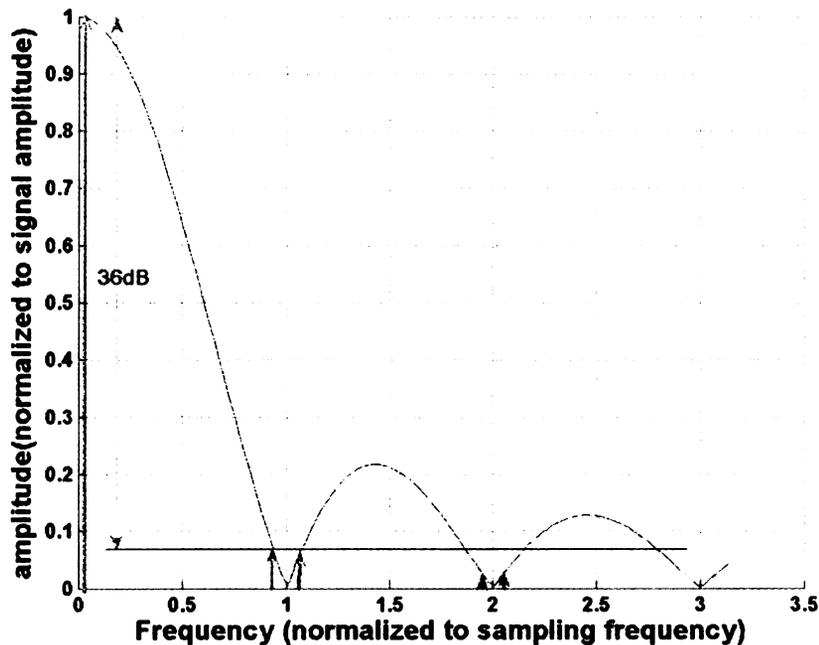
Figure 5.7. The spectrum of an R-chain DAC. The envelop is a rectified sinc function, the frequency is normalized to the sampling frequency, and the output amplitude is normalized to the signal strength.
