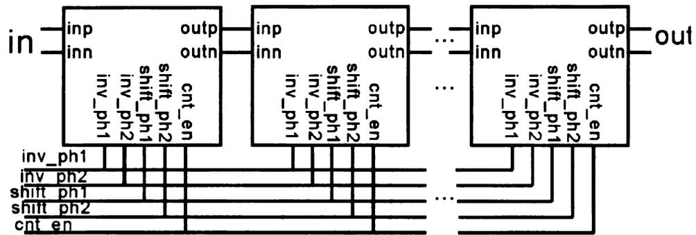
Figure 4.18. Block diagram of the scalable up/down counter.
