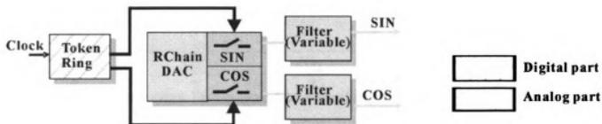
Figure 5.6. Architecture of a resistor chain DAC based quadrature sinusoid signal generator.
