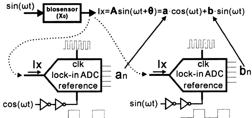
Figure 4.1. The lock-in ADCs extract and digitize the impedance information of a biosensor.
