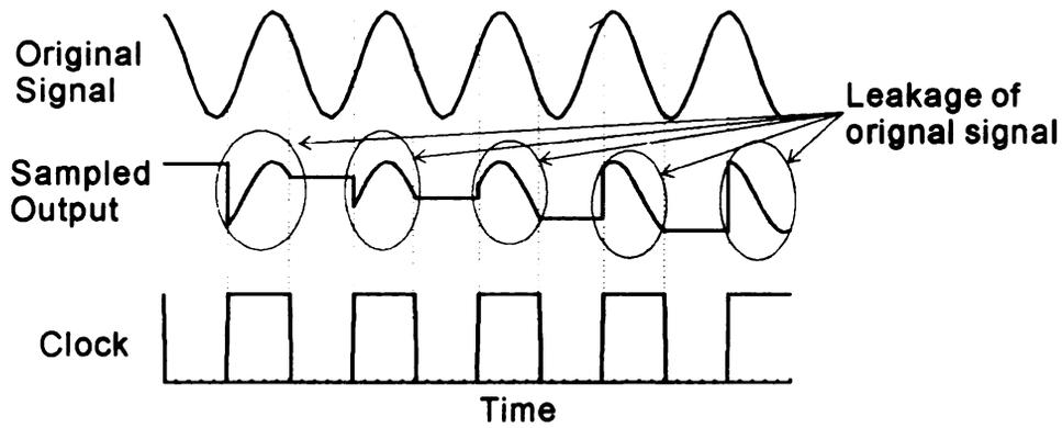
Figure 5.21. The original signal leaks out to the output through the tracking window.
