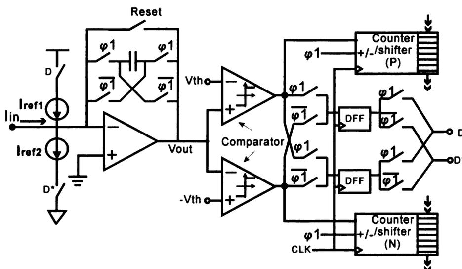
Figure 4.9. Block diagram of the lock-in ADC based IS system.
