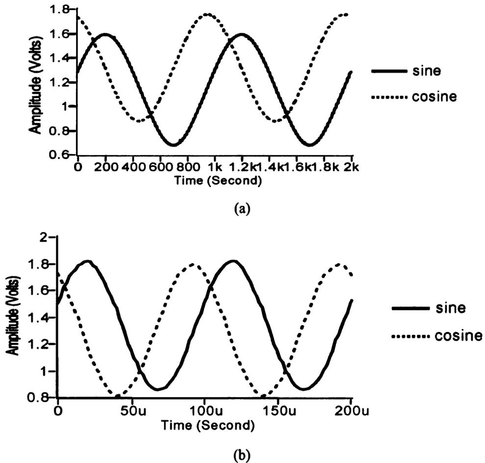
Figure 6.13. Waveform of quadrature sinusoid output at two extreme frequencies, (a) 1mHz and (b) 10KHz.
