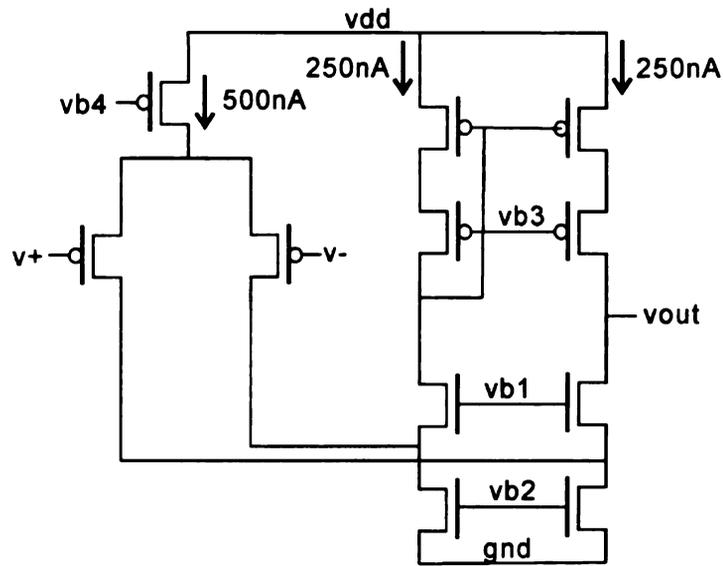
Figure 4.12. Folded cascade op-amp circuit designed for the lock-in ADC system.
