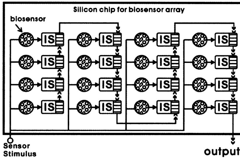
Figure 4.2. Block diagram of the biosensor array based microsystem.
