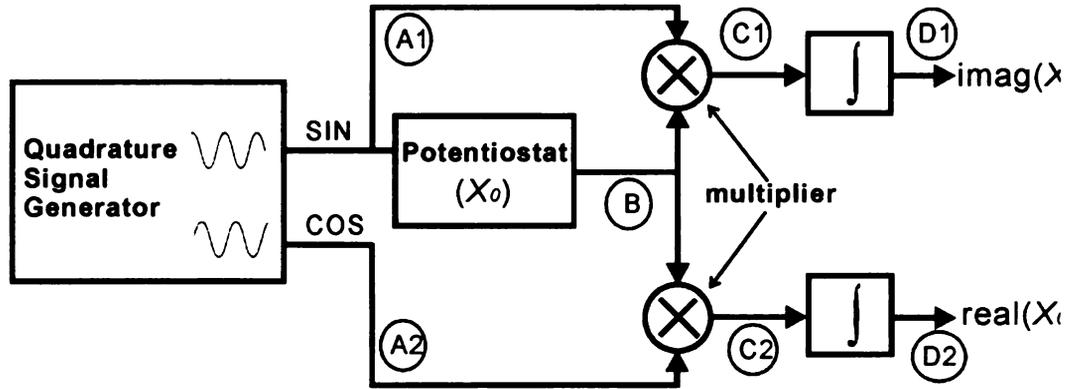
Figure 3.4. Block diagram of frequency response analyzer based impedance Spectroscopy.
