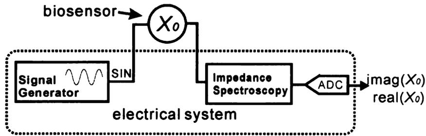
Figure 1.7. Electronic system of the impedance spectroscopy.
