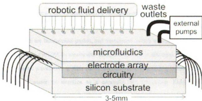
Figure 1.3. Integrated biosensor microsystem.
