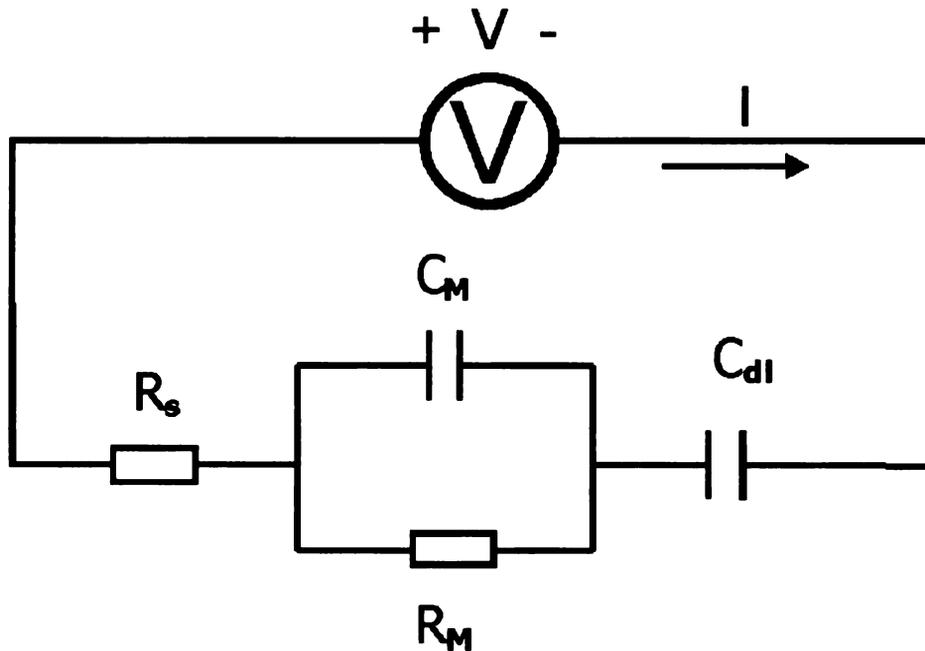
Figure 3.5. Equivalent circuit model for tBLM biosensor.
