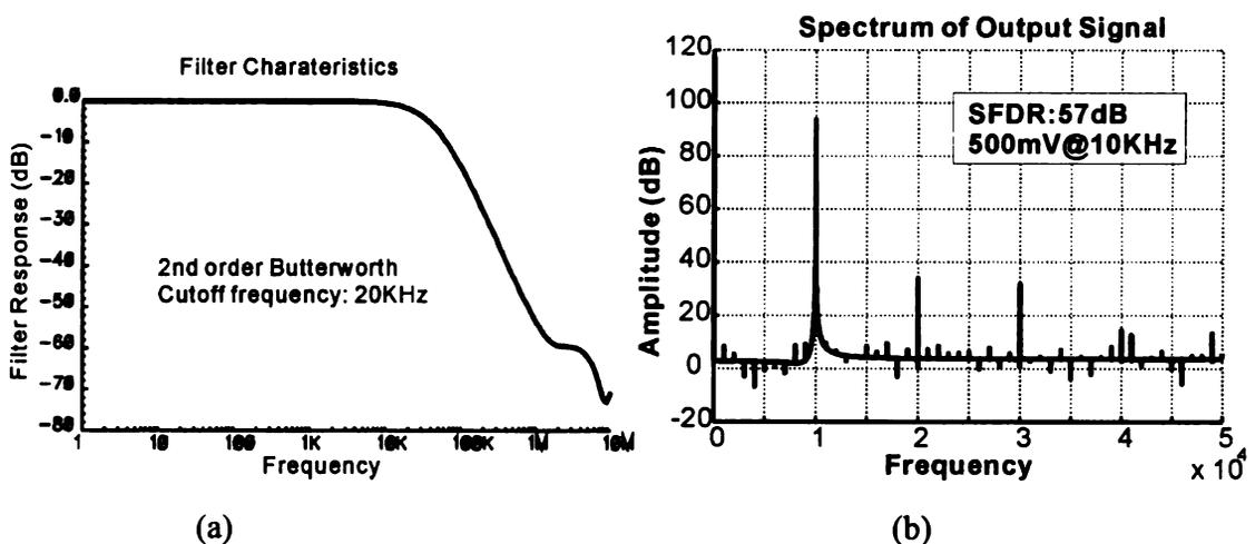
Figure 5.16. (a) Transfer function and (b) linearity of the variable filter with a cut-off frequency of 20KHz.
