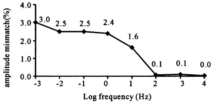
Figure 6.15. The amplitude mismatch between the output quadrature signals.
