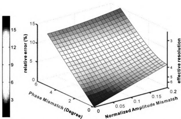
Figure 3.9. Output relative error versus the different levels of mismatch in amplitude and phase of two identical biosensors, and the equivalent resolution in terms of digital presentation.
