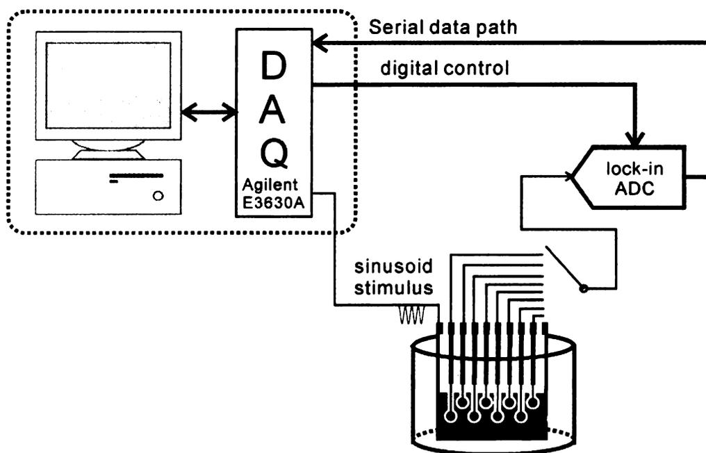
Figure 6.17. The experiment setup for the real biosensor impedance extraction.
