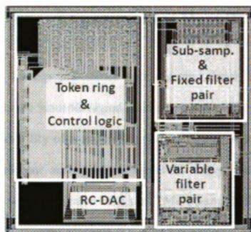
Figure 5.23. The layout of the quadrature sinusoid signal generator. Its size is  $1\text{mm}^2$ .
