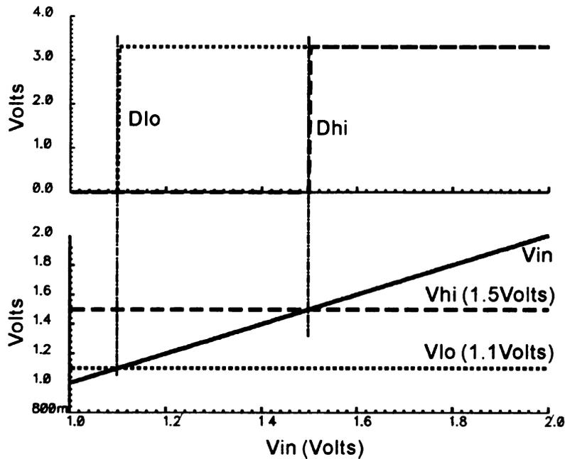
Figure 4.15. The input voltage DC sweep of the dual level comparator.
