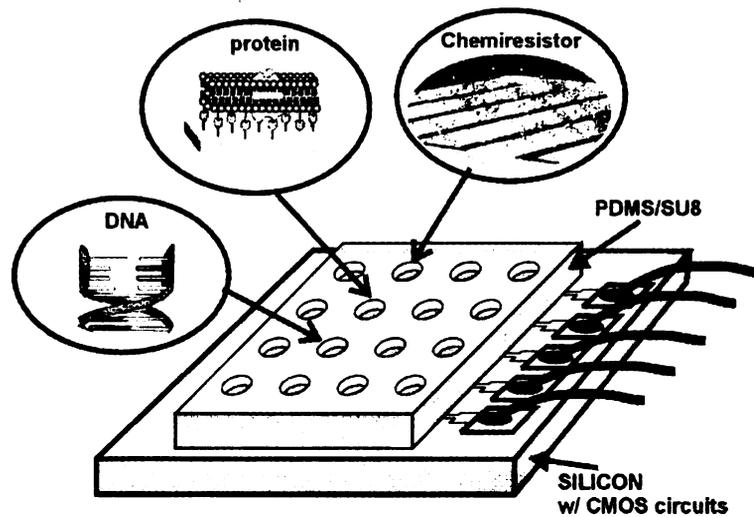
Figure 1.1. Concept diagram of the biosensor array microsystem, the miniaturized biosensor array is built on top of the integrated circuit die.
