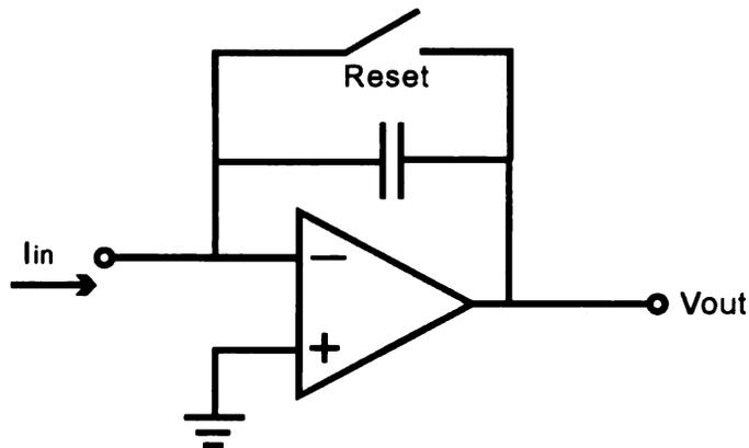
Figure 4.4. Simple integrator circuit.
