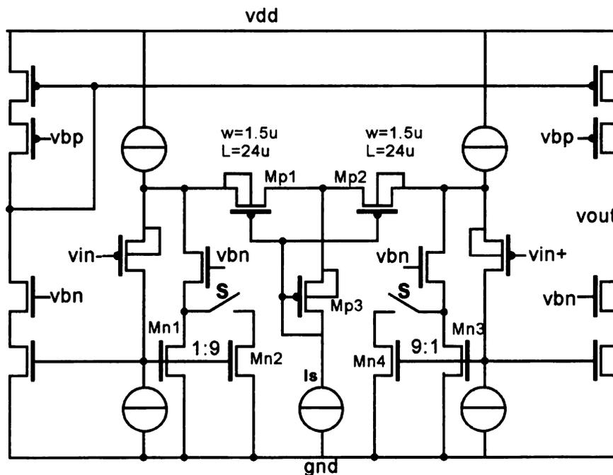
Figure 5.13. OTA with a small  $g_m$  (two level tunable). The signal S selects the  $g_m$  level.
