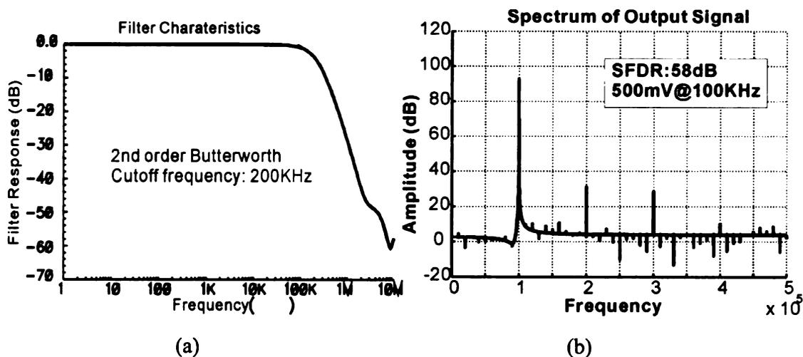
Figure 5.15. (a) transfer function and (b) the linearity of the variable filter with cut-off frequency of 200KHz.
