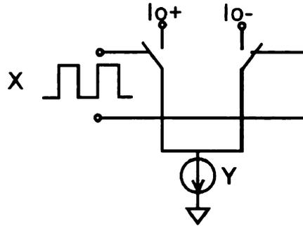
Figure 4.7. A simplified chopping circuit, Y is a current input, X is large square-wave signal.
