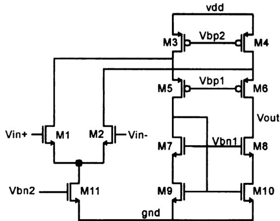
Figure 2.7. Schematic of the folded cascode OTA.
