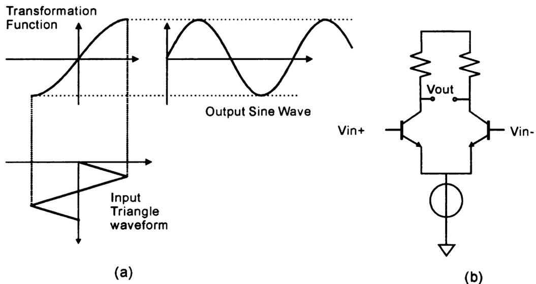
Figure 5.3. The principles of a triangle-to-sine signal generator: (a) transformation from triangle waveform to sine waveform, (b) a typical circuit to perform the transformation.
