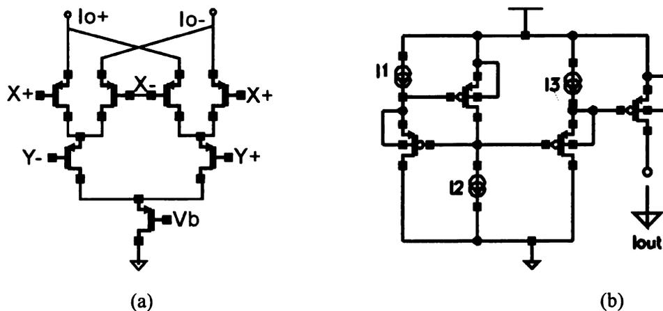
Figure 4.6. The subthreshold multiplier: (a) Gilbert subthreshold CMOS analog multiplier, (b) CMOS translinear principle based multiplier.
