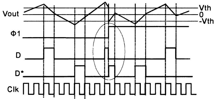
Figure 4.10. Waveform of the compensation current control signal ( $D$  and  $D^*$  in Figure 4.9), for  $D$  and  $D^*$  are low on the flipping of the capacitor.
