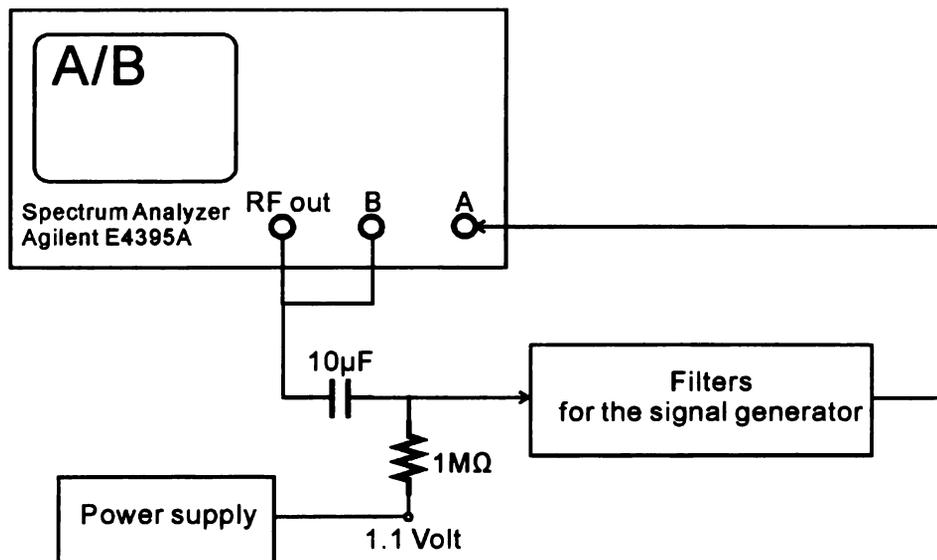
Figure 6.9. Experiment setup for the filter testing.
