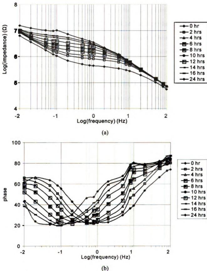
Figure 6.18. Impedance of monolayer and tBLM: (a) magnitude, (b) phase.
