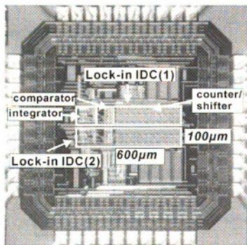
Figure 6.1. Die of two lock-in ADCs.
