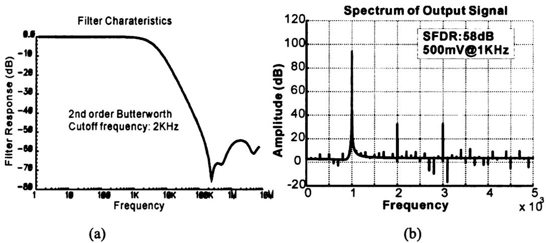
Figure 5.17. (a) Transfer function and (b) the linearity of the variable filter with a cut-off frequency of 2KHz.
