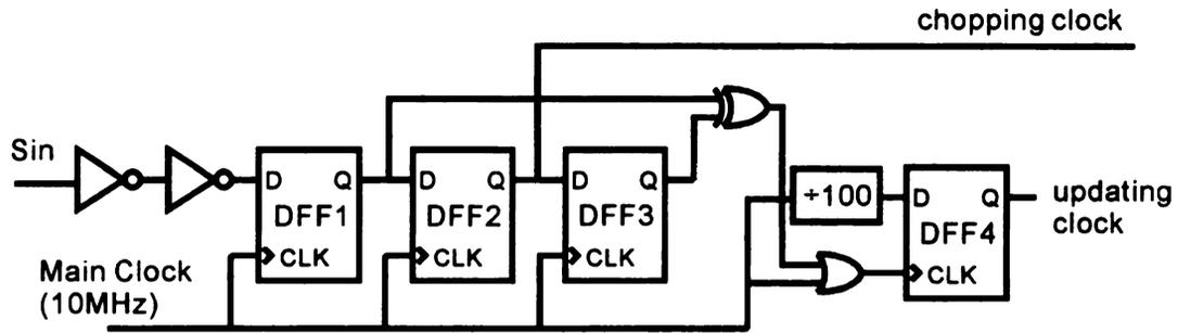
Figure 4.11. Block diagram of the control block, which generates the updating clock and the chopping control signal. An XOR gate is used to generate a pulse covering the edge of the chopping clock. This pulse will block the change on the updating clock through gating the clock of DFF4 and therefore avoiding conflict between the chopping signal and the updating clock.
