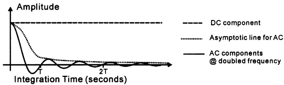
Figure 3.6. The DC and double frequency AC interference in the integrator output.
