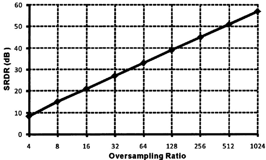
Figure 5.8. Linearity versus oversampling ratio for the DAC's output.
