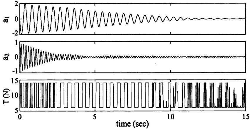
**Figure 6.14.** Plot of the modal amplitudes of the 1<sup>st</sup> and 2<sup>nd</sup> mode, and the control action (cable tension)
