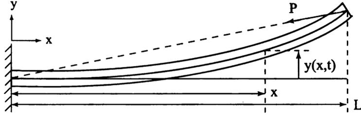
**Figure 6.1.** Cantilever beam with cable-supplied end force.
