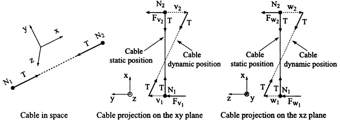
**Figure 6.6.** Cable element and its projections on the x-y and x-z planes
