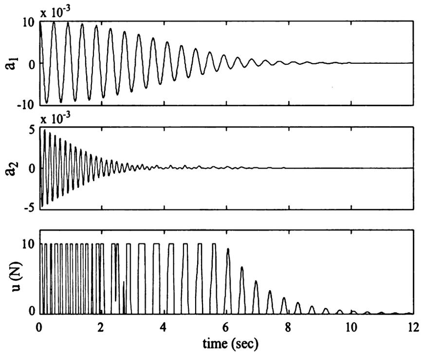
**Figure 6.12.** Plot of the modal amplitudes of the 1<sup>st</sup> and 2<sup>nd</sup> mode, and the control action (cable tension)
