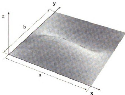
**Figure 5.4.** Uniform rectangular membrane fixed on all sides
