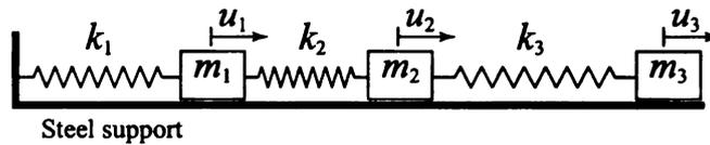
**Figure 5.1.** A three dof mass-spring system
