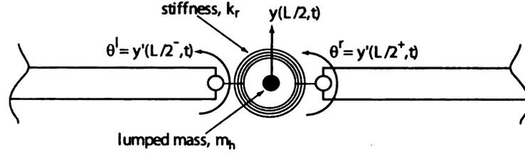
**Figure 3.2.** The hinge model
