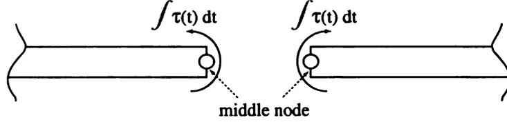
**Figure 3.3.** Action-reaction pair of impulsive moments
