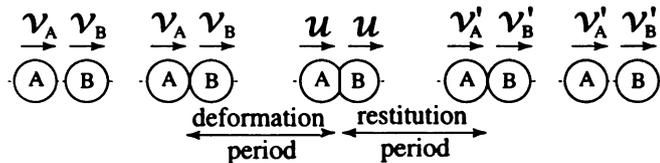
**Figure 4.2.** Direct central impact between two masses
