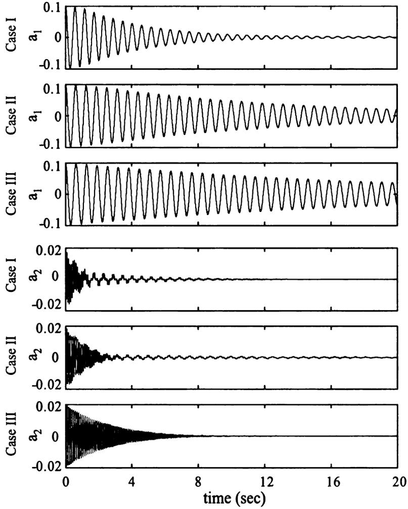
**Figure 6.4.** Simulation of decay in modal amplitudes  $a_1$  and  $a_2$  due to the control shown in Fig.6.2, for cable configuration in Case I (connection at  $x = L$ ), Case II ( $x = 3L/4$ ), and Case III ( $x = L/2$ ).
