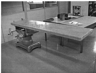
Figure 6.10 Custom examination table with a nonmetallic composite top that does not interfere with the applied magnetic field
