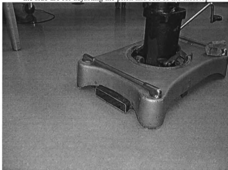
Figure 6.13 A bracket is welded underneath the base of the custom examination table for accommodating a wooden extension arm that provides additional support and stability.
