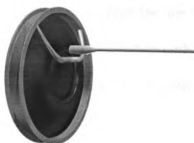
Figure 12.24 Optimal position of the gradiometer in relation to the outlet strut
