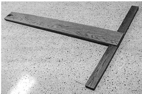
Figure 6.14 A T-shape wooden extension is used to increase the stability of the custom surgery table when in use
