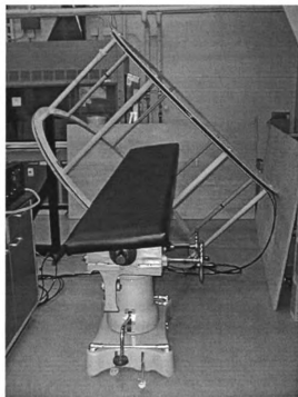
Figure 6.7 Custom examination table positioned between the excitation coils. The excitation coils system is designed to accommodate both the patient and the custom examination table.
