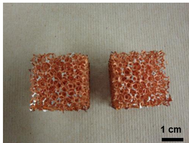
Figure 3.5 Top view digital image of Cu coated Al foams at cut area
