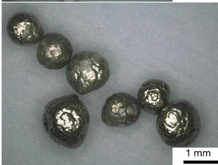
Figure 4.9 Visualization of Ni deposition on PE pellets. Non-PAH modified PE pellets were not able to form Ni coating.
