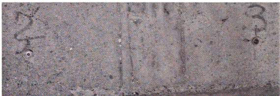
Figure 4-4 Measuring points with contact seats screwed on brass cylinders
