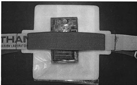
Figure 3.2. A photo of the accelerometer mounted on the custom acrylic plate and attached to the triathlon belts.
