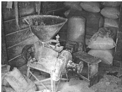
Figure 3.2 Milling machine (plate mill 2-A type) used by a custom miller in Ga East District
