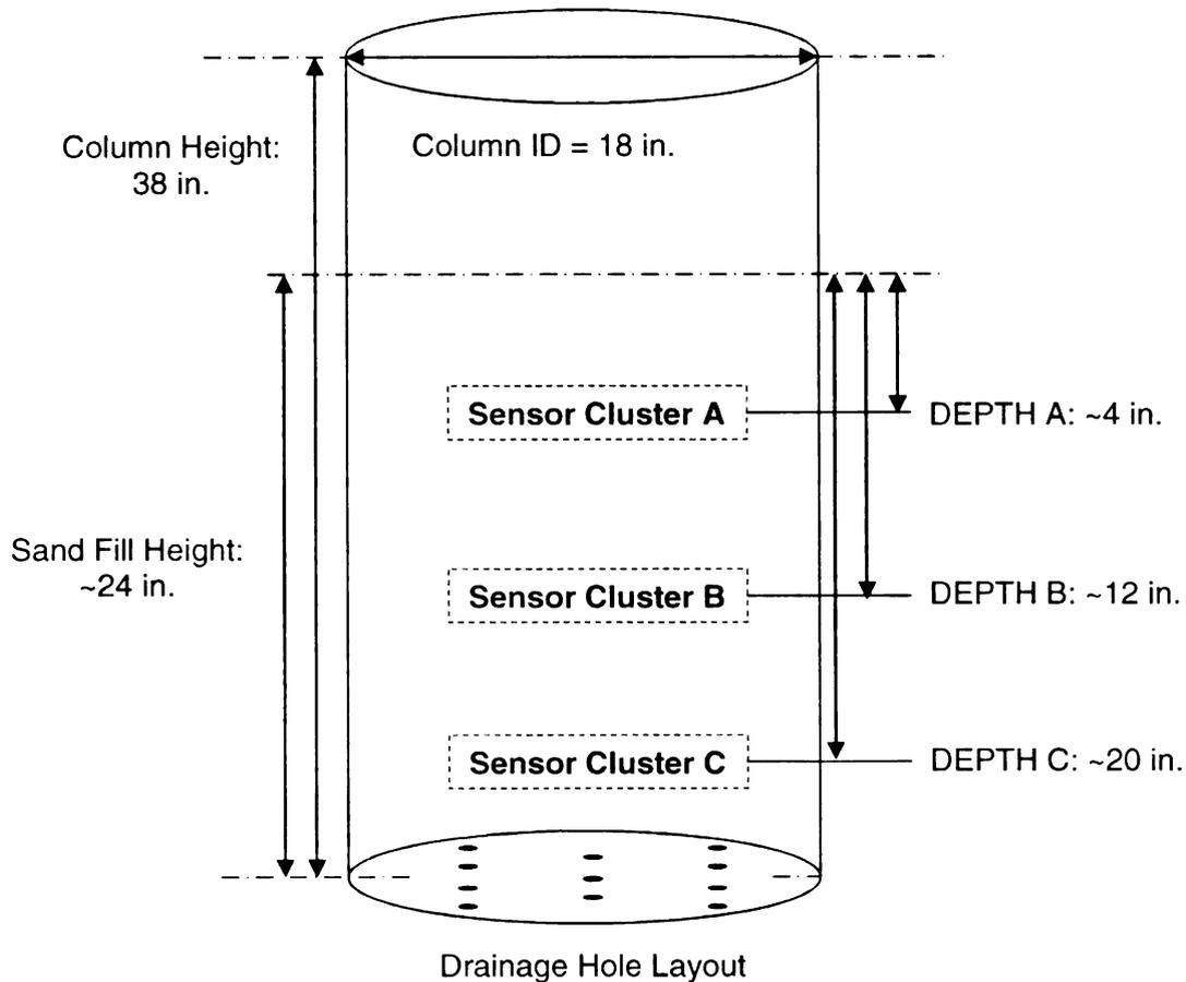
**Figure 2-4. Soil Column Dimensional Schematic with Drainage Holes**
