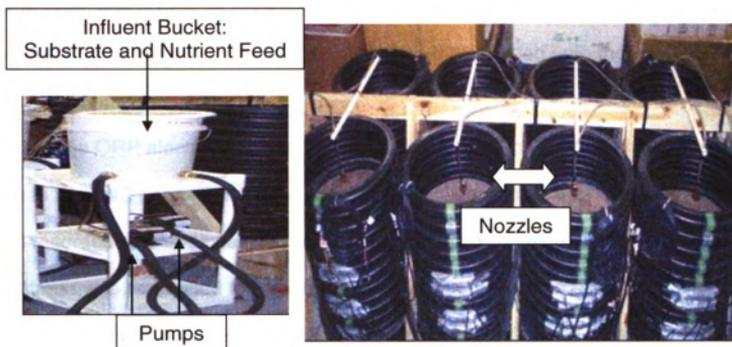
Figure 2-6. Substrate and Nutrient Feed and Column Set-up, Top View
