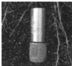
Figure 2-2. Oxygen Sensor (Model O2S-D) by Apogee Instruments Inc. (Bugbee and Blonquist 2007)
