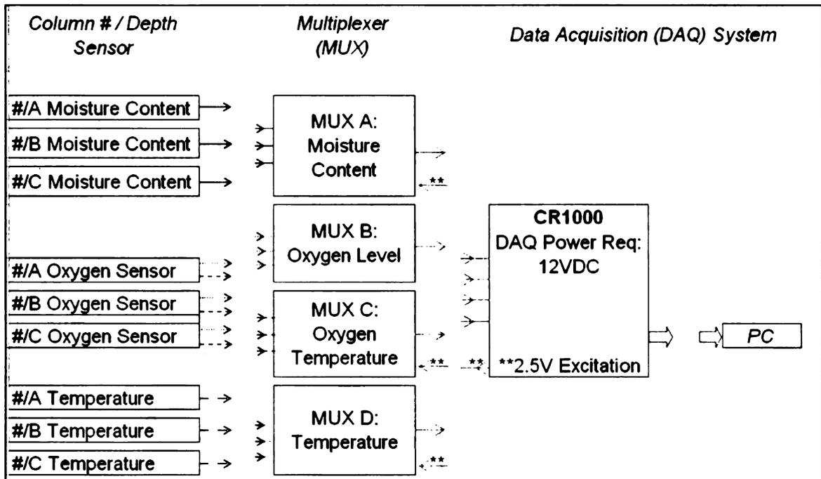
Figure 2-7. Basic Sensor Wiring Diagram
