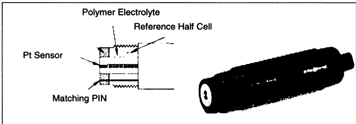
Figure 2-3. HI 2005-1005 ORP Probe and Schematic (Hanna Instruments)
