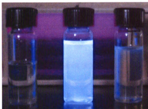
Figure 59. Reaction of 3-azido-7-hydroxycoumarin with polymer micelles. Vial 1: polymeric micelles and dye in the absence of “click” catalyst; Vial 2: polymer micelles and dye after the “click” reaction; Vial 3: dye and components for “click” reaction without polymer micelles.
