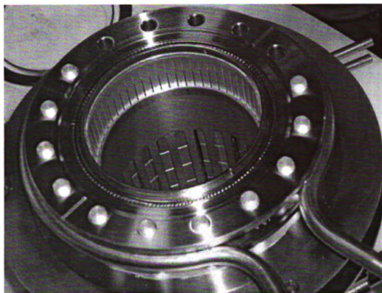
Figure 4.13. Assembled straight absorber device ready for installation. Here ceramic absorber tiles can be seen under copper coupling slots next to an array of bellows fingers.
