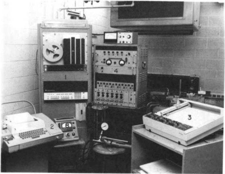
Figure 5.2.--Photograph of equipment set up for the foil gage technique. Minicomputer (1), teletype (2), X-Y recorder (3), 6-channel amplifier (4), bonded specimen (5), coldworking apparatus (6), hydraulic pump (7), Bridge Amplifier Meter (8).
