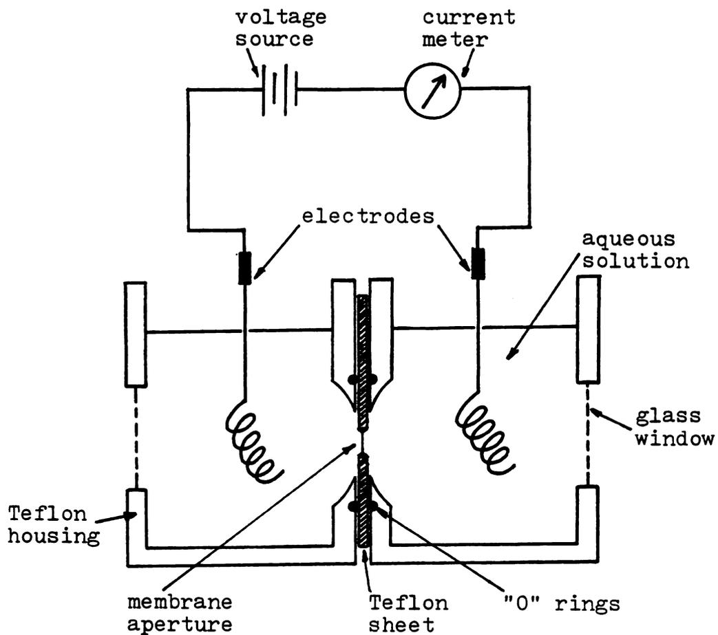
Figure 1-3. Cell for the electrochemical study of bilayer lipid membranes.
