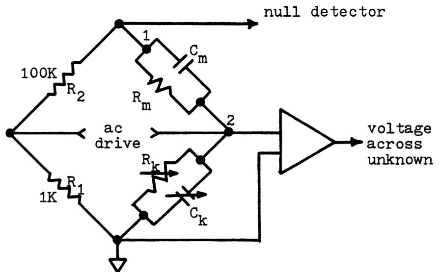
Figure 1-5. A simplified ac bridge circuit (by S. H. White) for the measurement of membrane capacitance.
