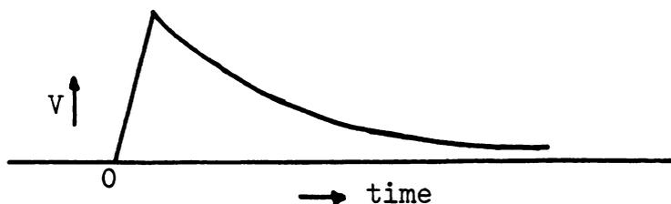
Figure 1-7(c). An idealized voltage decay.
