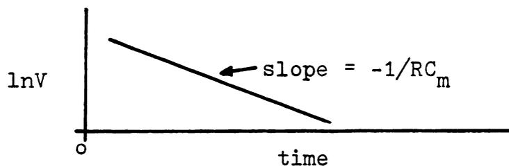
Figure 1-7(d). A  $\ln v$  versus  $t$  straight line. If  $(R_f + R_s) \ll R_{\text{ext}}$ ,  $R = 2(R_f + R_s) + R_{\text{ext}} \approx R_{\text{ext}}$  and the membrane capacitance can be obtained from the slope.
