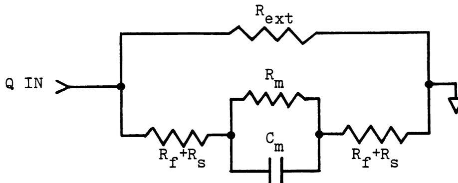
Figure 1-7(a). Equivalent circuit when an external resistor is placed across the membrane between two electrodes.
