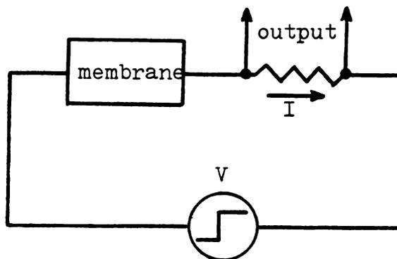
Figure 1-6. A schematic circuit for the measurement of the membrane capacitance by the dc transient method.
