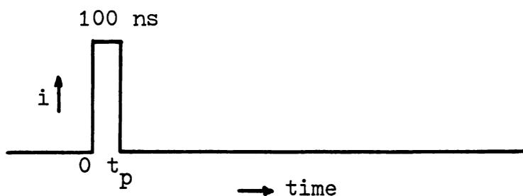
Figure 1-7(b). A short constant current pulse.  $Q_{\text{total}} = it_p$ .
