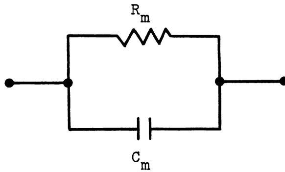
Figure 1-4. A simplified, equivalent circuit of an unmodified bilayer lipid membrane.
