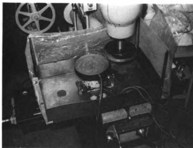
Fig.18. Soil sample prepared before test
