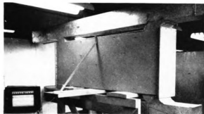
Fig. 36 Laboratory test arrangement for plate-type heat exchanger
