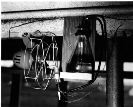
Fig. 50. A continuous wet bulb instrument built according to plans by Henderson. Both a dry and wet thermocouple are in the fan air stream.
