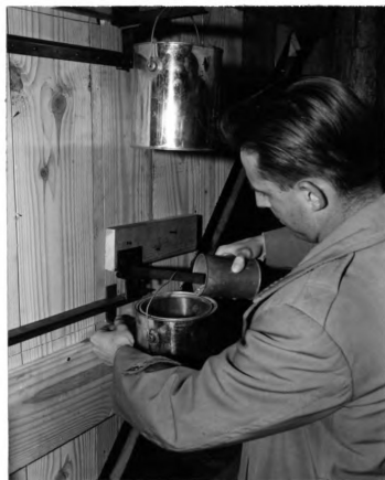
Figure 21. Lateral Pressure Test Showing Peeler Gage.
