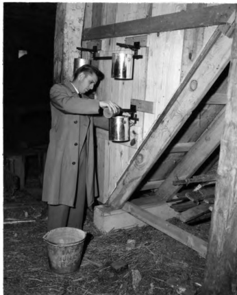
Figure 19. Apparatus for Making Lateral Pressure Tests.
