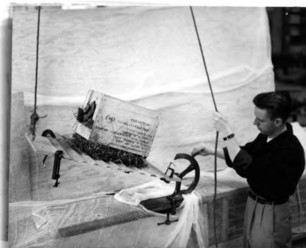
Figure 24. Apparatus for Measuring Coefficient of Friction Showing Quadrant Lock.
