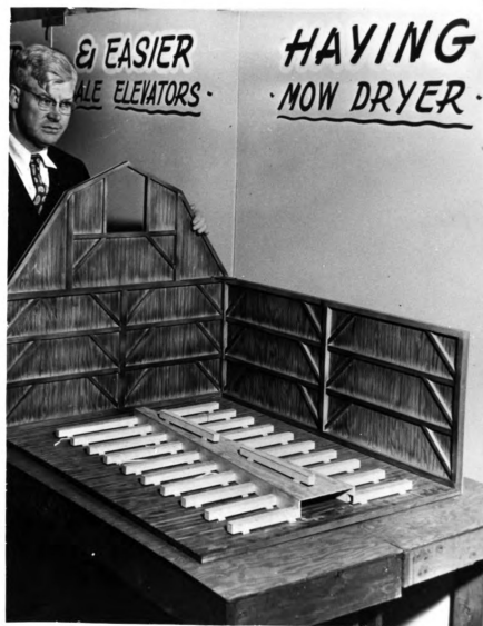
Fig. 43. A model of a mow hay drier. Air is forced through the central tunnel by means of a fan. The side tunnels give equal distribution of the air through the mow. (Courtesy: Michigan State College)
