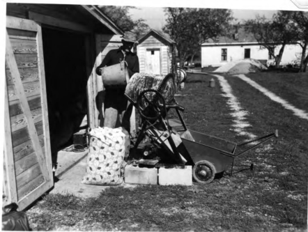
Fig. 64. A portable motor may be used in operating a concrete mixer. (Courtesy: "Northern Illinois Farm Life" magazine.)
