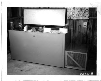
Fig. 15. A frozen food unit for a farm home. The motor driver compressor is shown at the right. (Courtesy: Michigan State College)
