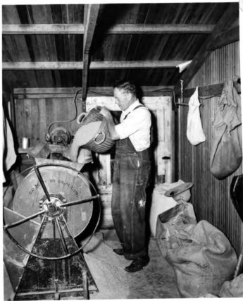
Fig. 28. An electric feed mixer on a Northern Illinois farm. (Courtesy: "Northern Illinois Farm Life" magazine)
