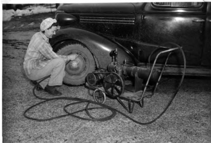
Fig. 63. A farmer's wife in Northern Illinois uses a portable electrically driven pump to inflate her tires. (Courtesy: "Northern Illinois Farm Life" magazine.)
