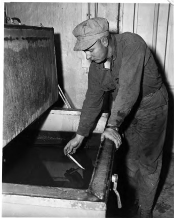
Fig. 31. An electric milk cooling tank for a dairy farm. (Courtesy: "Northern Illinois Farm Life" magazine)
