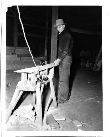
Fig. 65. An electrically operated circular saw suitable for farm uses. (Courtesy: "Northern Illinois Farm Life" magazine.)
