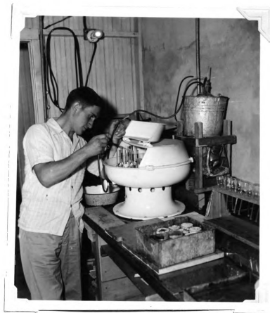
Fig. 35. Electricity is used in testing the percentage of butter fat in milk. (Courtesy: "Northern Illinois Farm Life" magazine)
