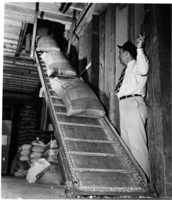
Fig. 41. An electric elevator for elevating bags of feed. (Courtesy: "Northern Illinois Farm Life" magazine)
