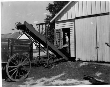
Fig. 42. An Illinois farmer loading a wagon with corn by using an electrically operated elevator mounted on wheels. (Courtesy: "Northern Illinois Farm Life" magazine)
