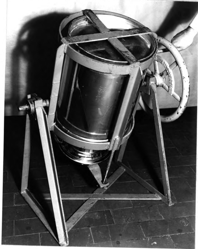
Figure 5. Constructed mechanical shaking apparatus showing method of rotating.
