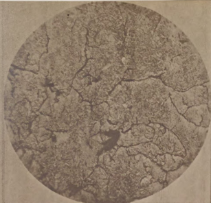
Etched, 1600° F, Magnification - X400 Constituents - Graphite, Martensite, Cementite
