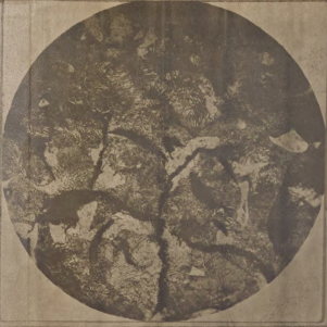
Etched - Untreated Magnification - X400 Constituents - Graphite, Pearlite, Ferrite
