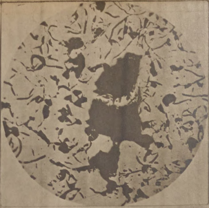
Unetched - 1700° F. Magnification - X100 Constituents - Graphite
