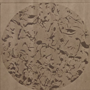
Unetched - 1600° F Magnification - X1100 Constituents - Graphite
