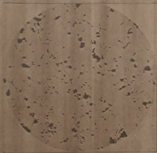
Unetched - 1400° F Magnification - X1100 Constituents - Graphite
