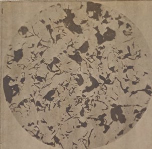
Unetched - Untreated Magnification - X100 Constituents - Graphite
