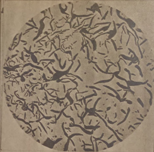
Unetched - 1800° F Magnification - X100 Constituents - Graphite
