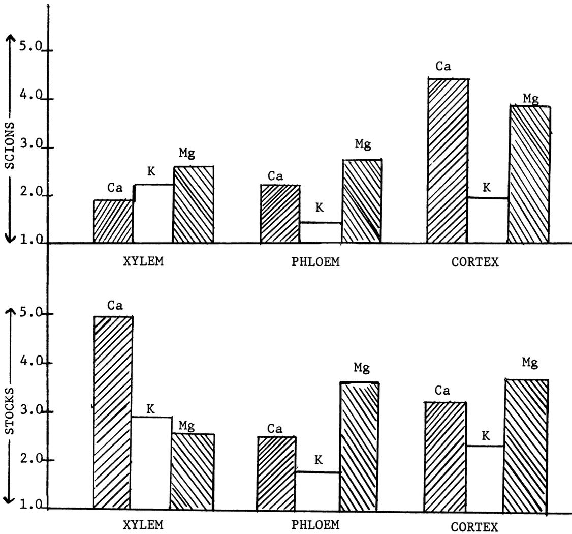
Figure 2. Mean calcium, potassium and magnesium content of interclonal juniper graft tissues within stock and scion as measured by electron microprobe X-ray analysis.
