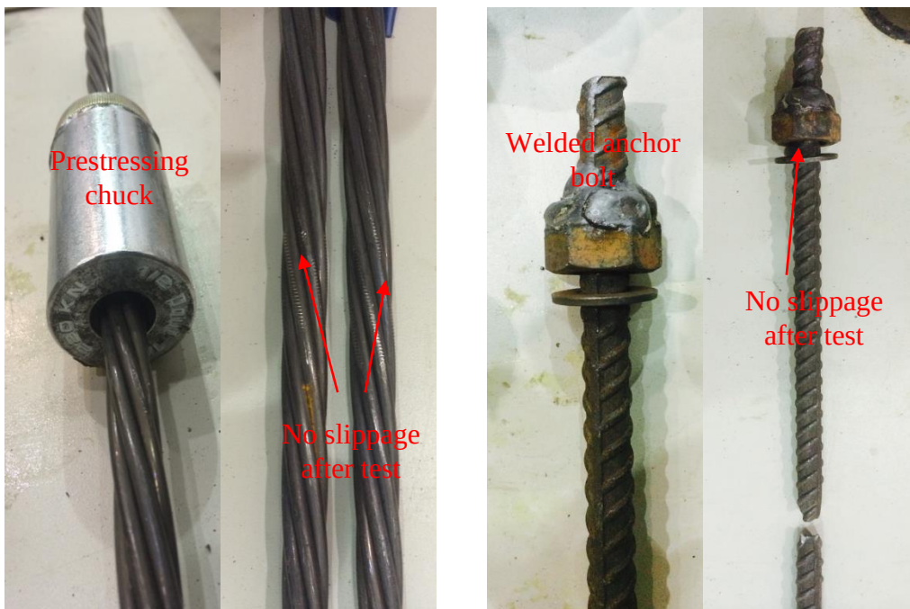
a. Chucks for prestressing strand b. Welded anchor bolts for reinforcing bar
