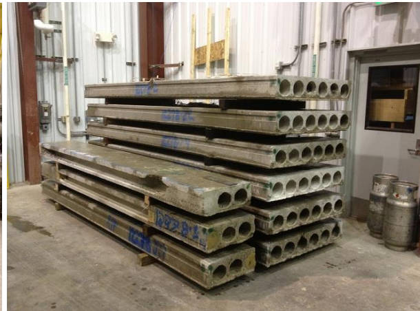
b. PC hollowcore slabs set for curing
