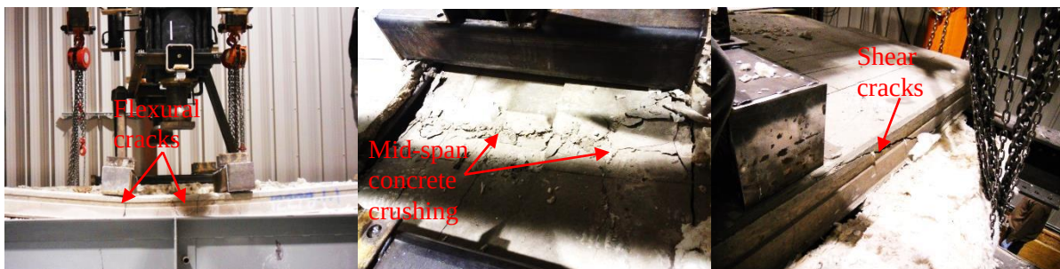
g. Slab 5, flexural cracks h. Slab 5, mid-span crushing i. Slab 6, shear cracks
