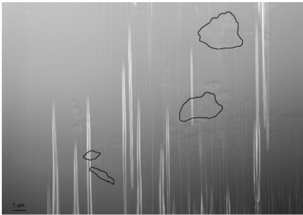
Figure 3.17: FESEM image of GnP dispersion in rigid PUR/PIR foam with 8 wt% pMDI treated GnP(750). Strut was prepared with the FIB and aggregates are outlined in black.
