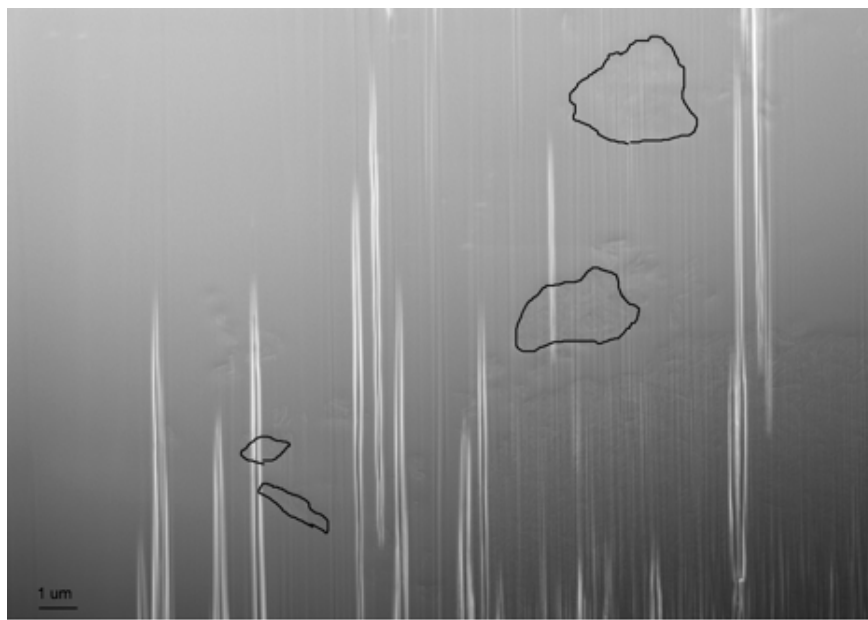
Figure 4.15: FESEM image of GnP dispersion in rigid PUR/PIR foam with 8 wt% pMDI treated GnP(750). Strut was prepared with the FIB and aggregates are outlined in black.
