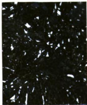
Time is very important and one second at 800°F. or one minute at 600°F. is as good a retained austenite decomposer as 40 to 60 minutes at 450°F. It should be noted here that just heating through the higher temperature ranges tends to rapidly decompose the retained austenite. Whether this decomposition is a matter of stress relief or carbon movement is beyond the scope of this paper. However either would be possible in the range of temperatures used.
