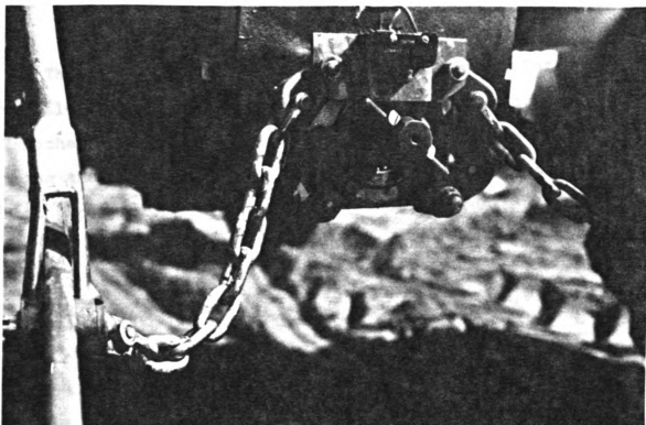
Figure 22. Microswitch indicating theoretical travel
