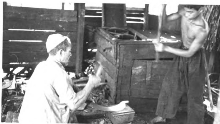
Figure 35. Blacksmiths making a tajak in Negara, Kalimantan shop
