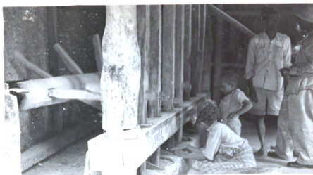
Figure 72. Interior of North Sumatra rice pounding mill showing wooden shaft and studs for lifting wooden hammers
