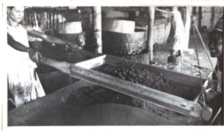
Figure 84. Screening brown sugar in East Java
