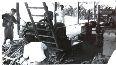
Figure 82. Horizontal roller power driven sugar mill in East Java
