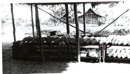
Figure 88. Small rubber processing shed with aluminum coagulating pans in South Sumatra
