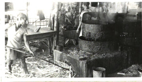
Figure 83. Circular iron inserts used to prevent juice foaming out of pan
